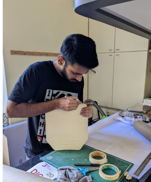
fig. 44 creasing and cutting from the edges to make the master
