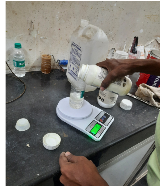
fg.39 Mixing resin in 3:1 ratio
