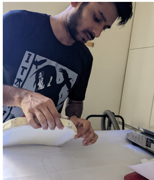
fig.43 masking the HAP mold with masking tape for making master pattern
