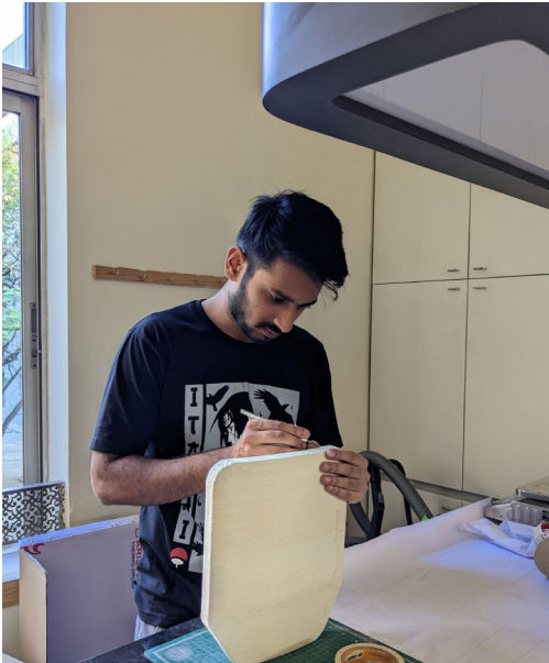
fig. 44 creasing and cutting from the edges to make the master
