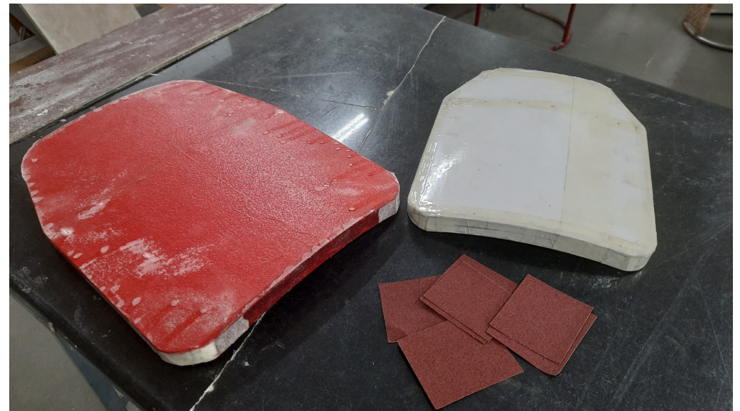
fg.41 sanding and finishing HAPs
