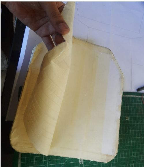
fig. 45 removing the masking tap layer
