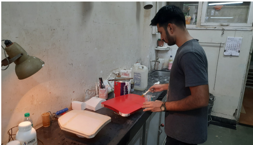
fg.40 applying resin to achieve smooth surface for pattern making
