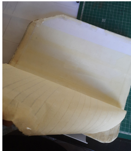
fig. 45 removing the masking tap layer
