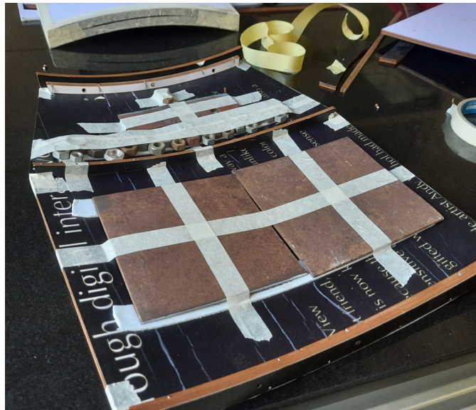
fig.37 Adding metal weight to mimic actual HAP weight
