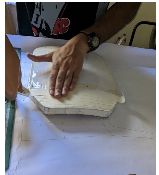
fig.43 masking the HAP mold with masking tape for making master pattern
