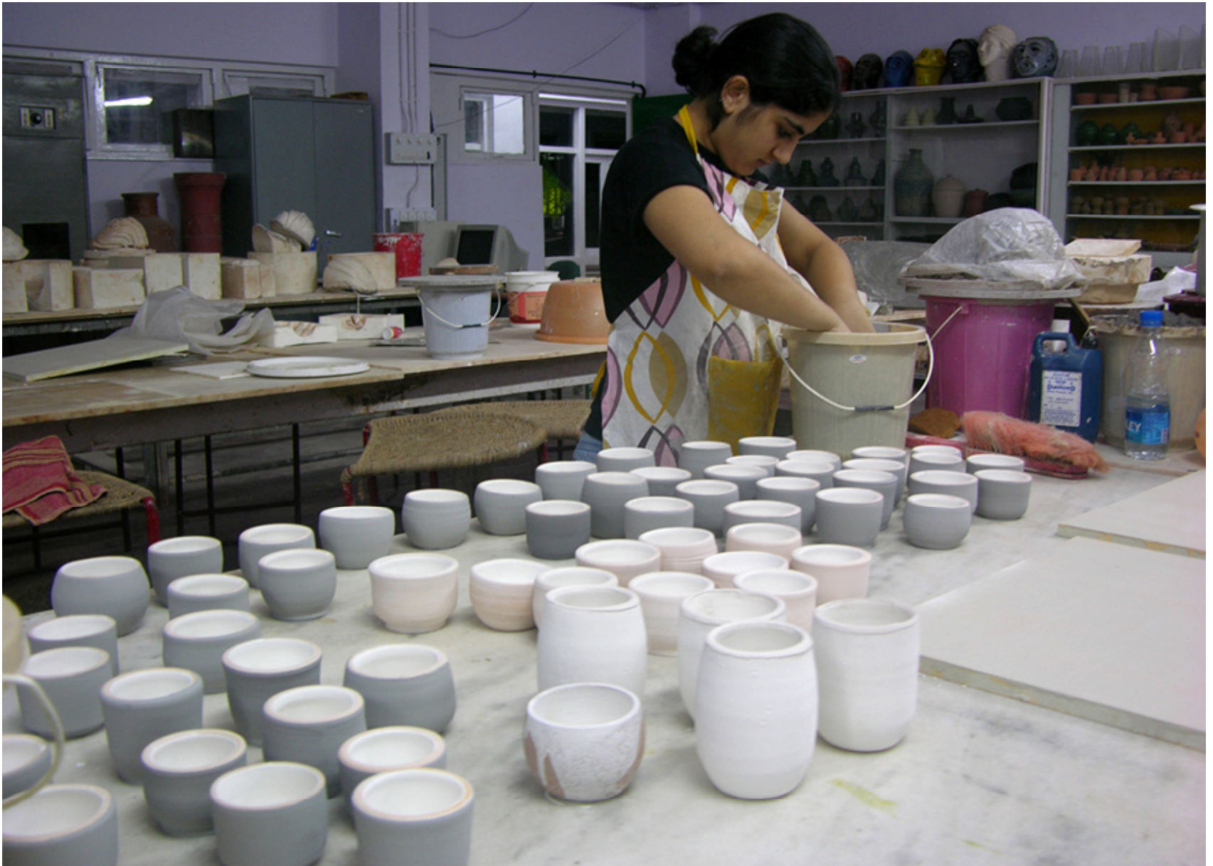
Dipping and pouring glazes on teacups (manganese and clear)
