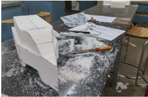
Img 63. Rough thermocol model as base for clay.
