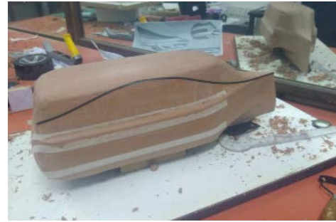
Img 65. Masking and planing.
