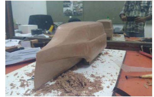
Img 66. Rough finish of clay model
