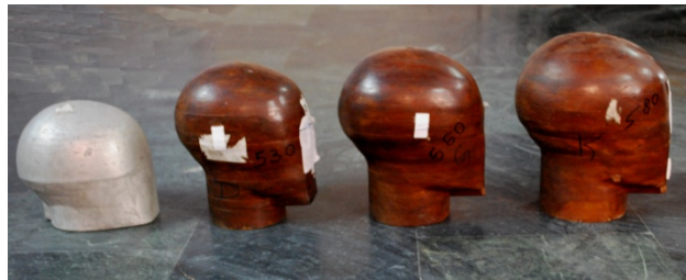
Standard head-forms for testing
