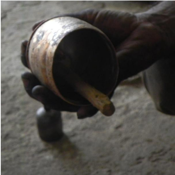
Attaching the wooden clapper on the bell
