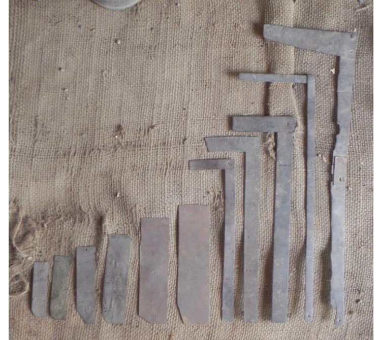
Standard measurements of babris and topics of a range of bell numbers
