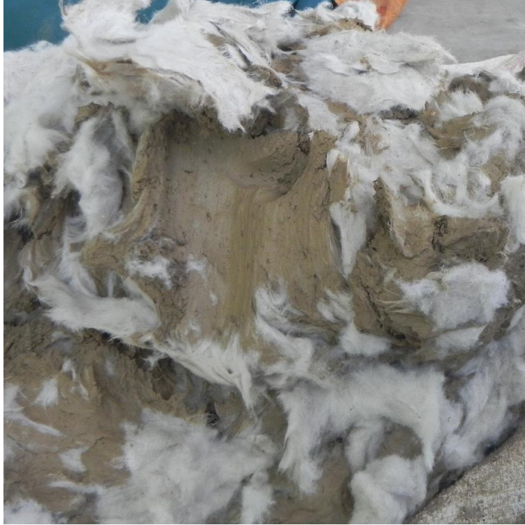
Cotton and mud mixed together using power hammer to get a uniform mixture dough
