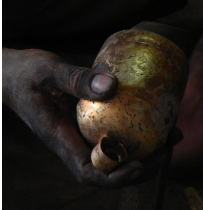
Making a Sound ring (crease) at a distance of about 10-15mm from edge
