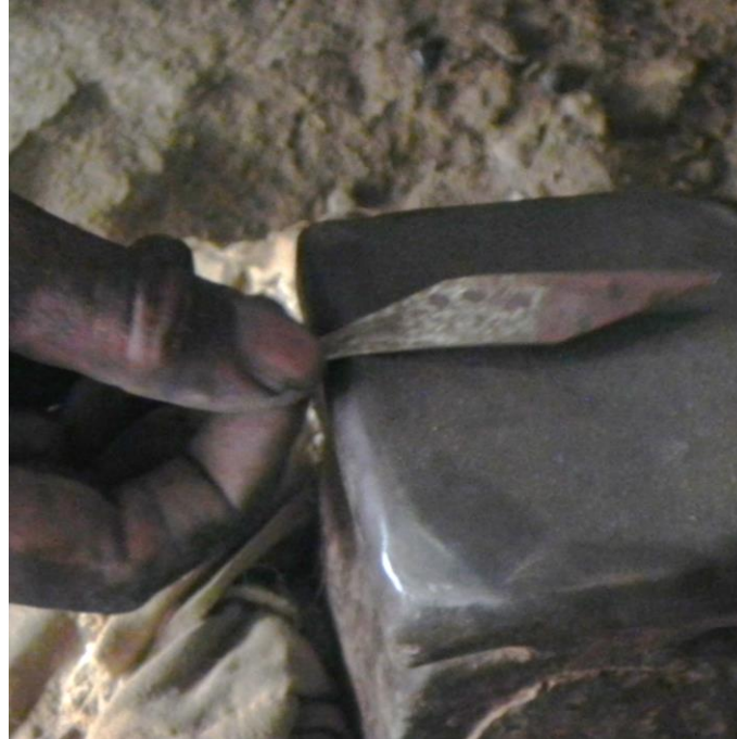
Hammering it on edges to get larger thickness and strength
