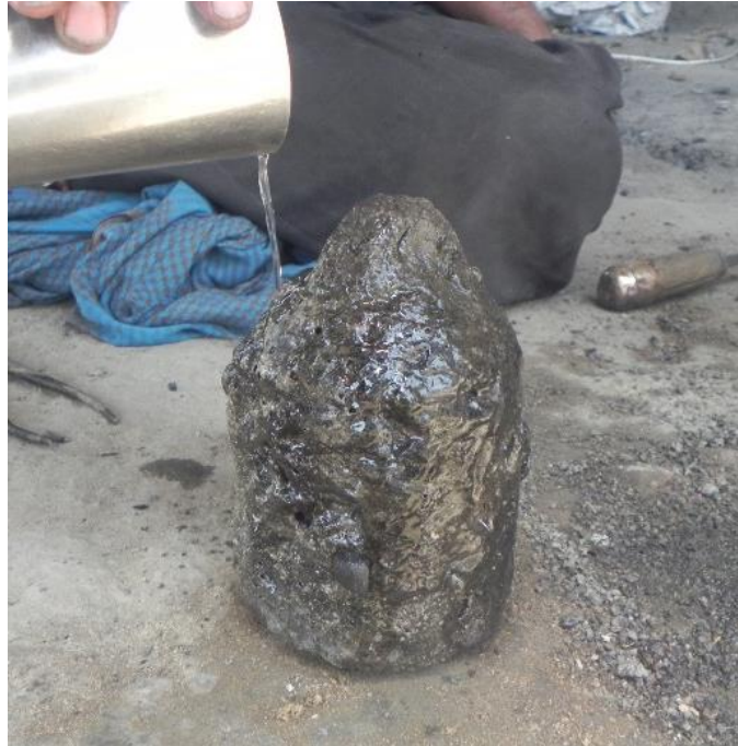
If it is still hot, pouring water onto it to cool the bell down
