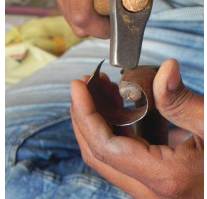
Shaping it into cylindrical form by hammering it on cylindrical end of tool
