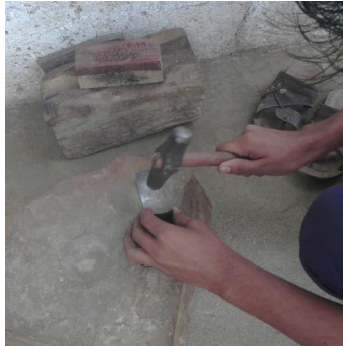
Shaping by hammering on a stone mold using round hammer
