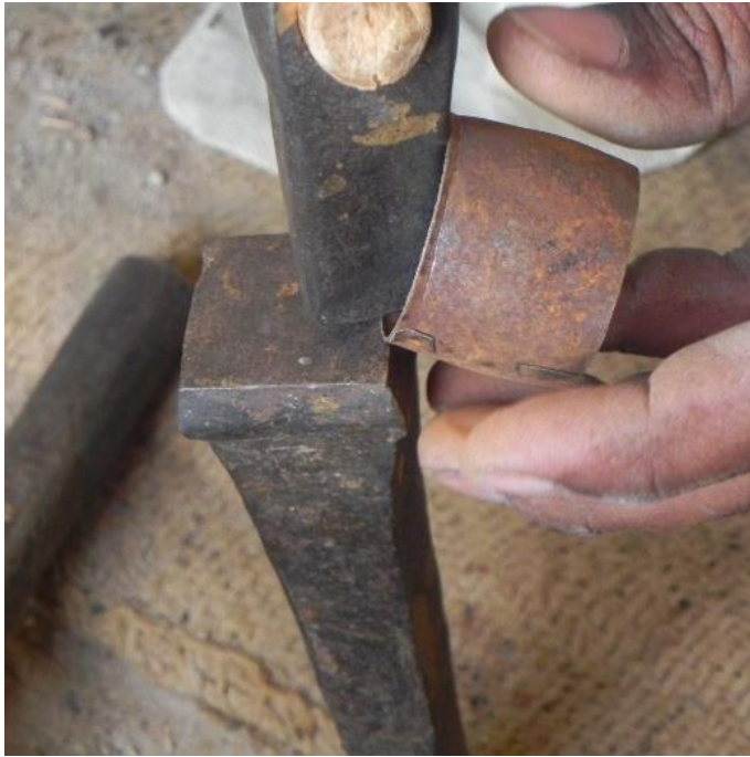
Thinning of one side of the edge of babri
