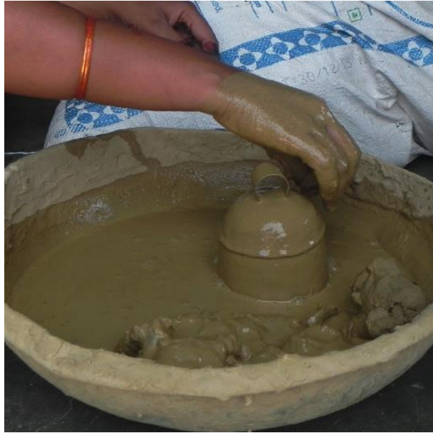
Dipping the bell into clay slurry just so that its surface becomes wet
