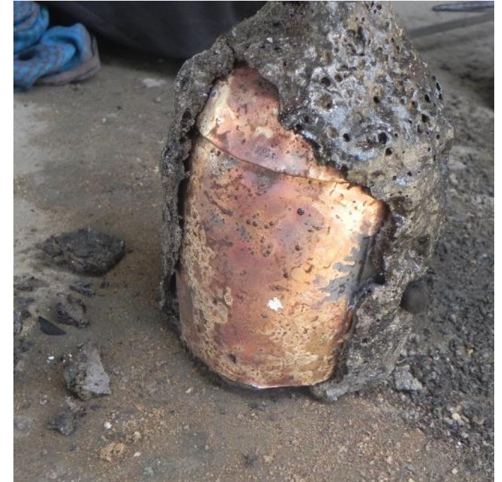
Cracking open the bell coating
