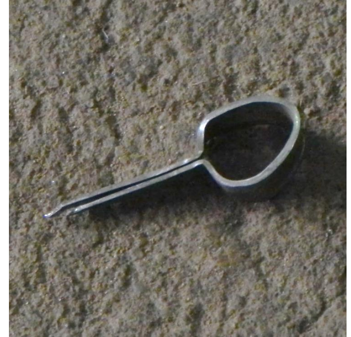
Shaping the sheet into circular hook shape
