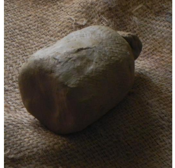
Mud coated bell ready for firing
