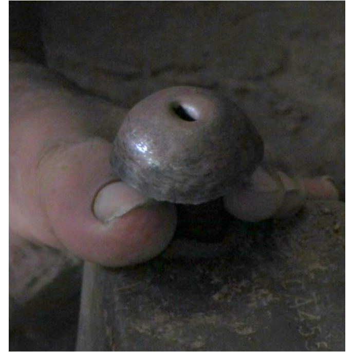
Making a hole in the topi (Space for putting kadi)
