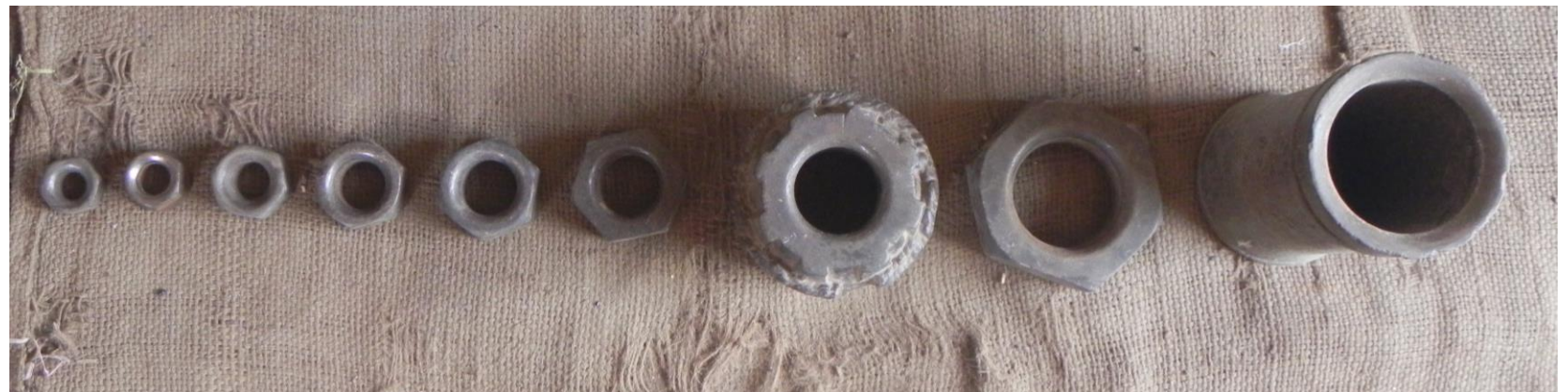
Nuts are used as a mould for making topics
