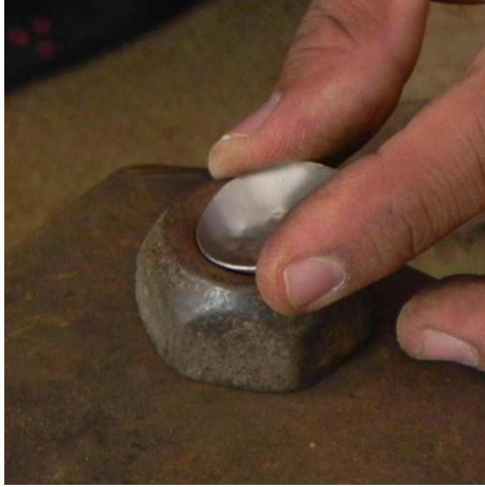
Hammering it to get hollow hemispherical shape
