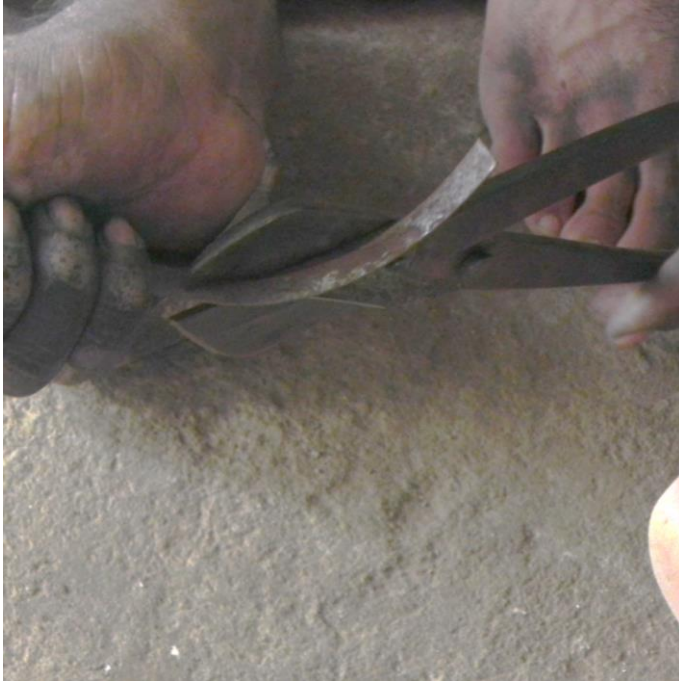
Cutting the kadi from MS metal sheet
