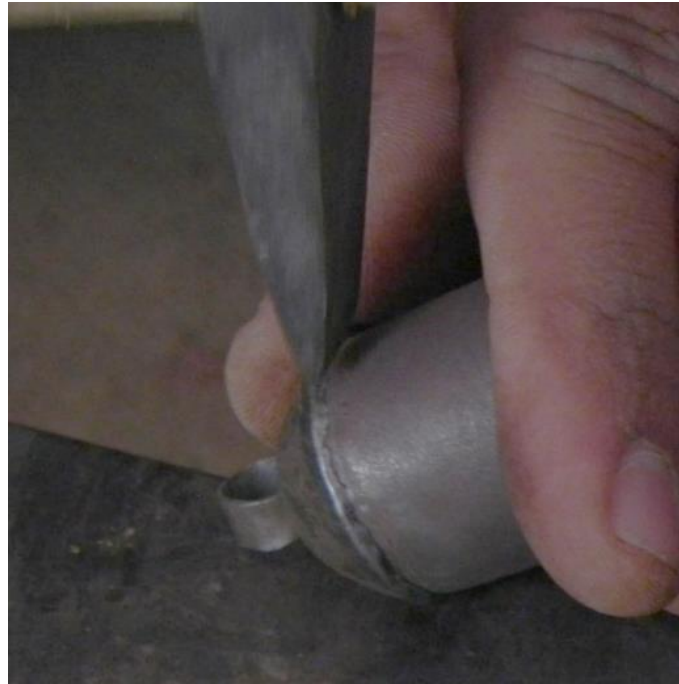
Locking the ends of hook by diverging them from inside
