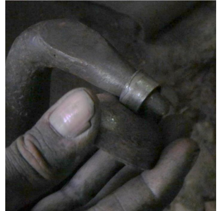
Shaping the hook to form proper circular ring
