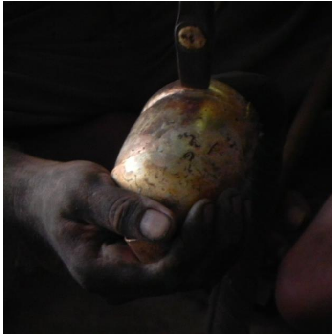
Hammering the crease and checking the sound
