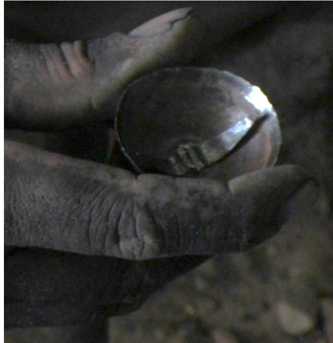
Locking the ends of hook by diverging them from inside
