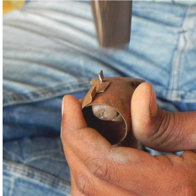
Technique to lock the notch
