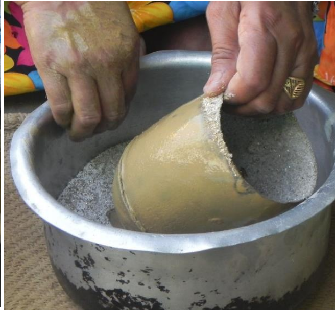
Sprinkling the brass mixture on wet slurry dipped bell
