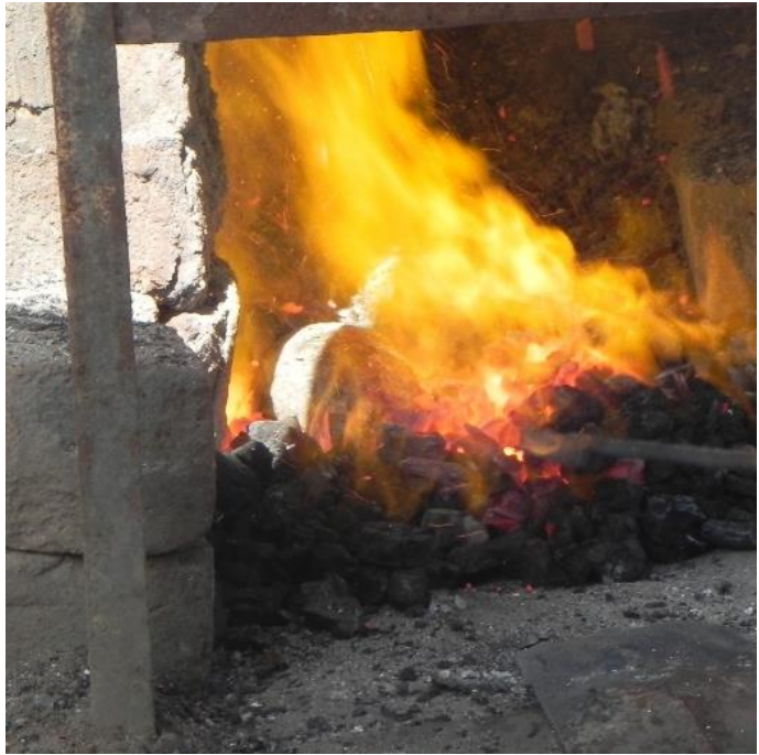
Putting the clay covered bell into the furnace to bake
