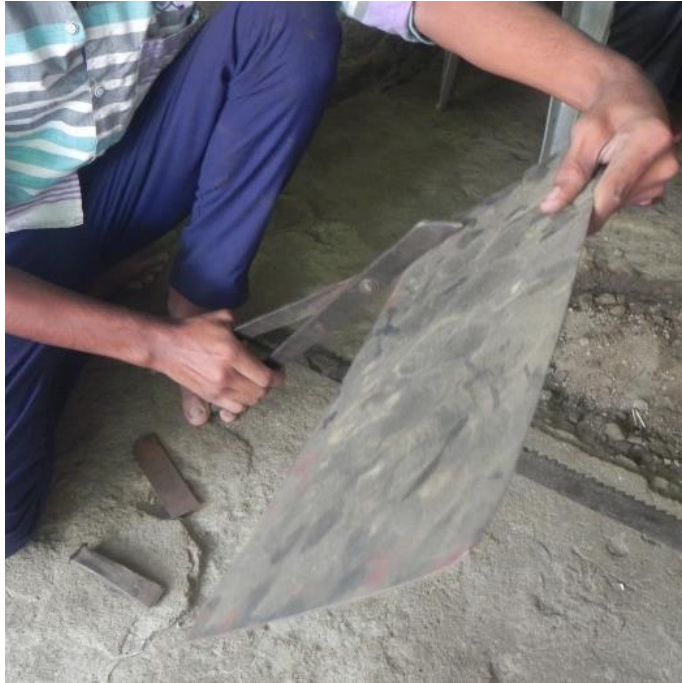
Cutting the MS Sheet into the rectangular shape according to size guide
