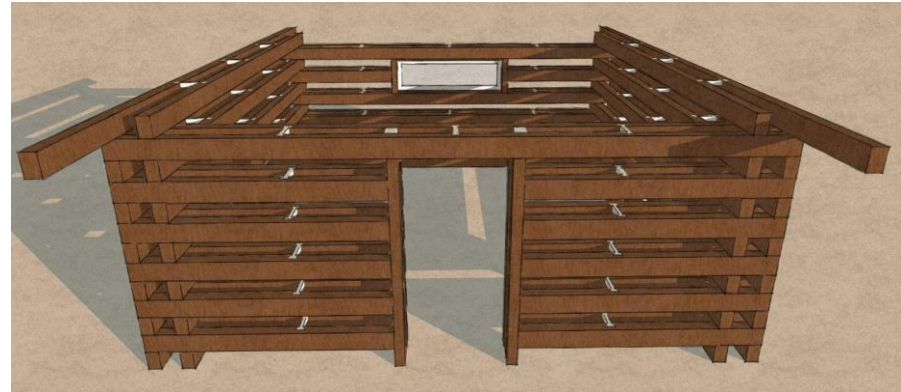
Fig 37: Traditional Kath-kuni wall timber laying pattern
