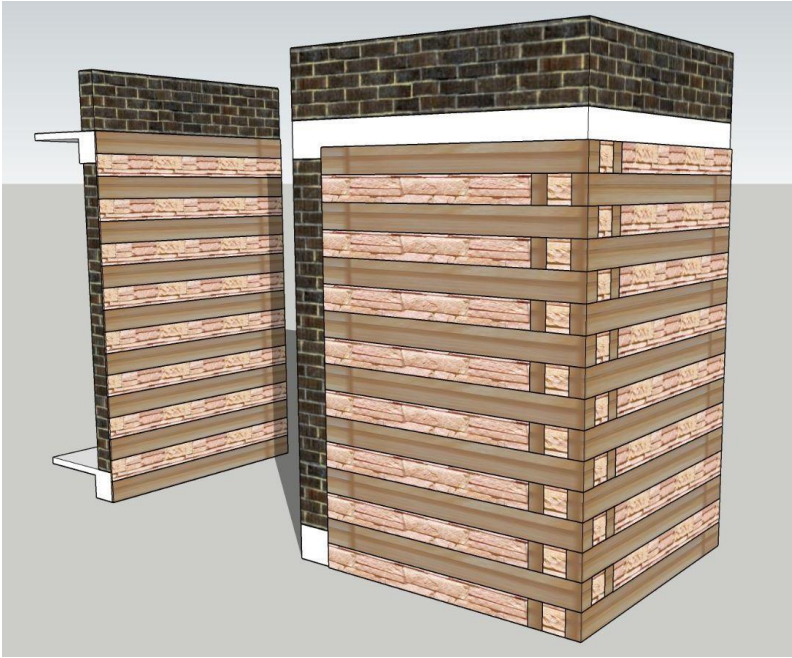
Fig 36, 37 Hybrid Kath-kuni wall laying pattern
