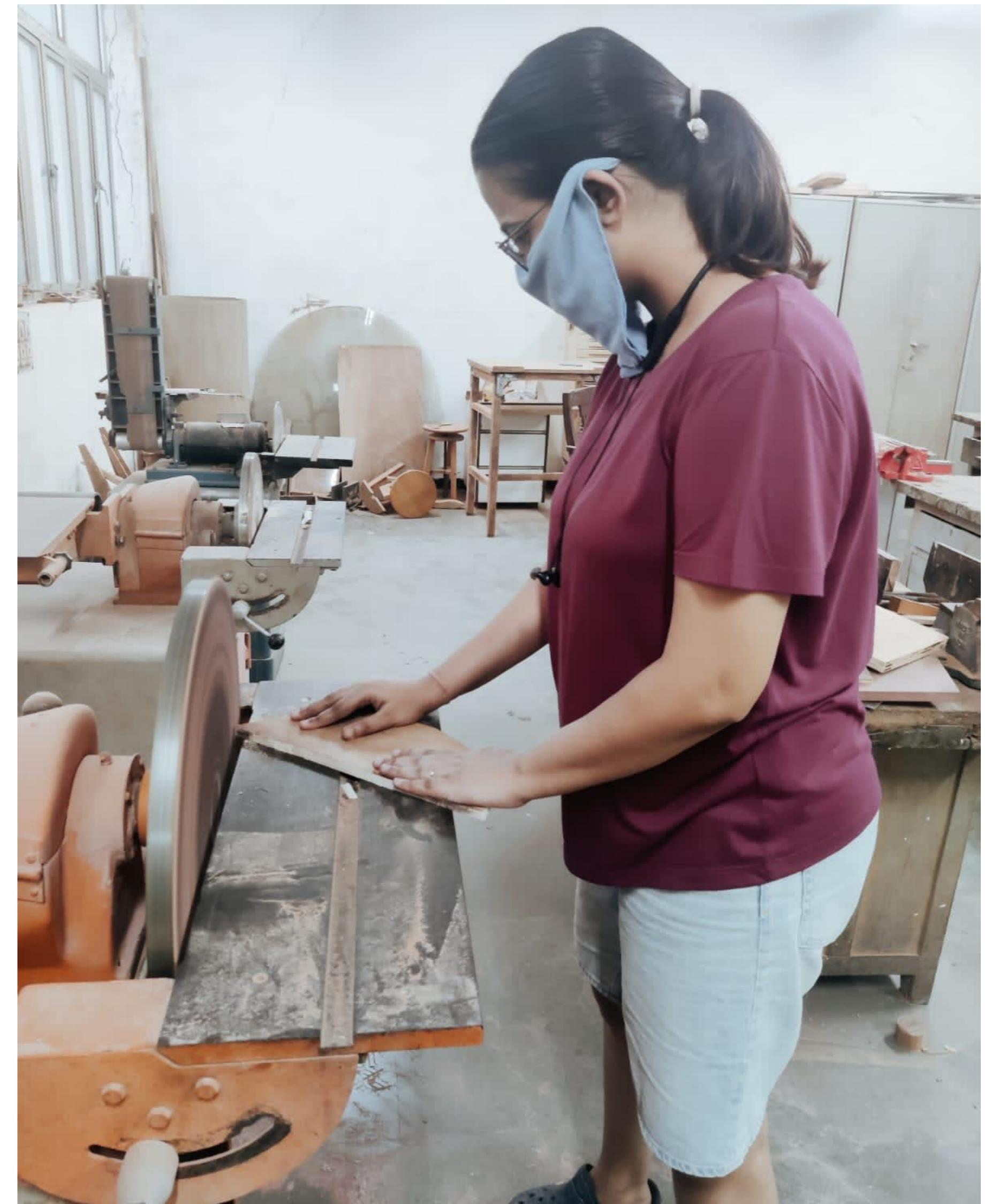
*Fig. Sanding the edges for smooth corners*
