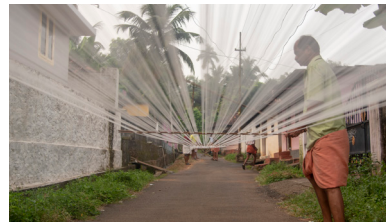
Warping is the process which converts the hank yarn into a linear form. The task requires many hands and each weaver is helped by his neighbours.
