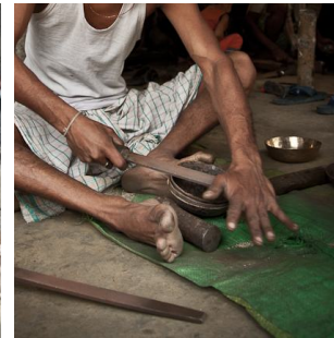
The edges are then filed or trimmed to desired length
