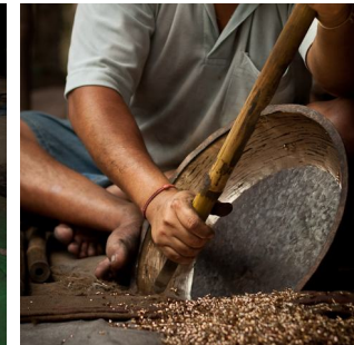
The soot is then scraped off for the bell metal to shine
