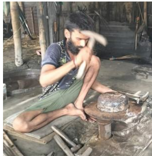
The disc is then heated & beaten to transform into desired shape
