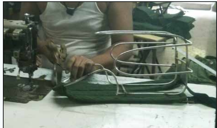
Fig 6.16: Canvas harness being stitched onto the metal frame
