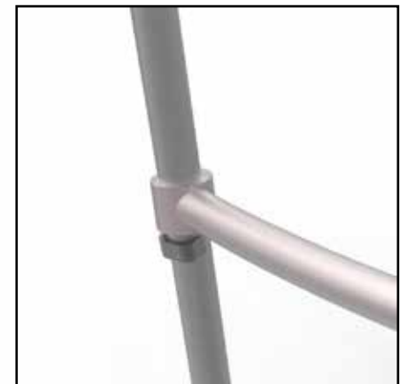
Fig 6.14: Side frame joint to main frame
