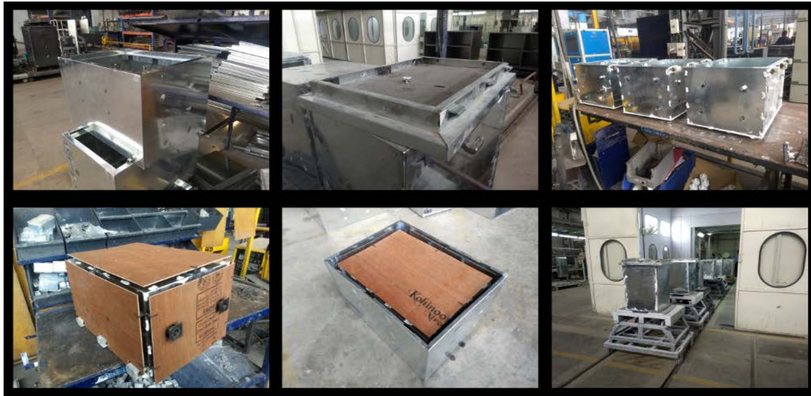
Figure 2.10 Pictures of fire resistant safe taken in the plant assembly line showing internal details.
