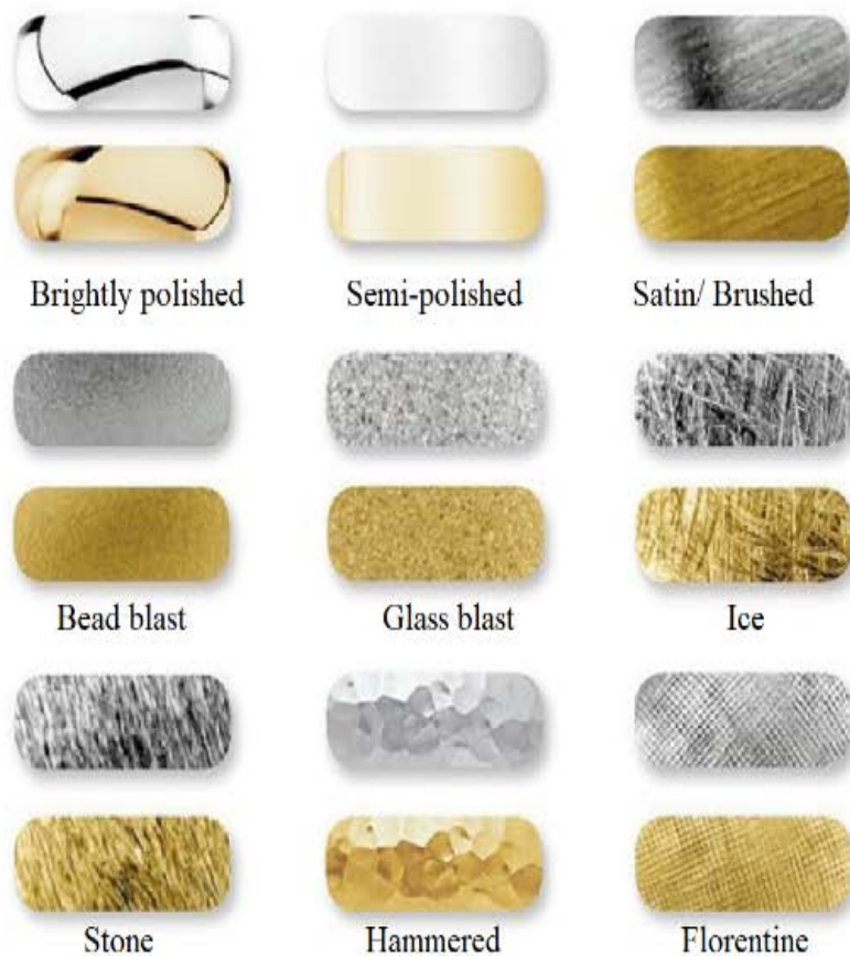
Figure 3.19 Types of material finishes we can use. It's the true material finish
