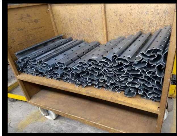
Figure 2.4 Metal sections used in the wall of safes
