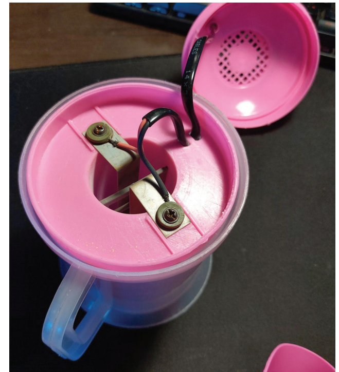
The two metal inserts are separated by a small plastic part and connected to main electricity connection. The whole system thereafter submerged to water for steam production.
