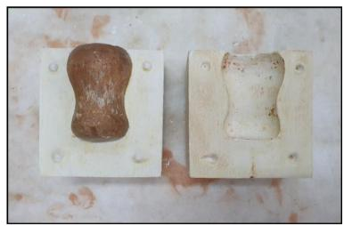
The form was made out of EPS. It was set on the marble counter and covered upto half height with clay an inch thick.
