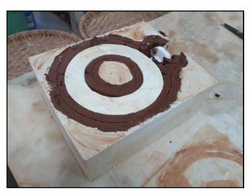
Once the plaster set the clay was removed and the entire thing coated in release again for the second batch of plaster to go in.
