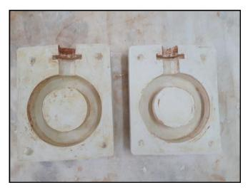
Had to wait a week for the mold to dry completely before the slip could be poured in.
