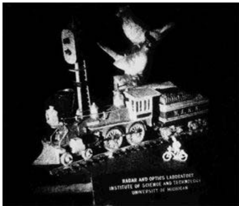
'Train and Bird' is the first hologram ever made with a laser using the off-axis technique. This pioneer image was produced in 1964 by Emmett Leith and Juris Upatnieks at the University of Michigan only four years after the invention of the laser
