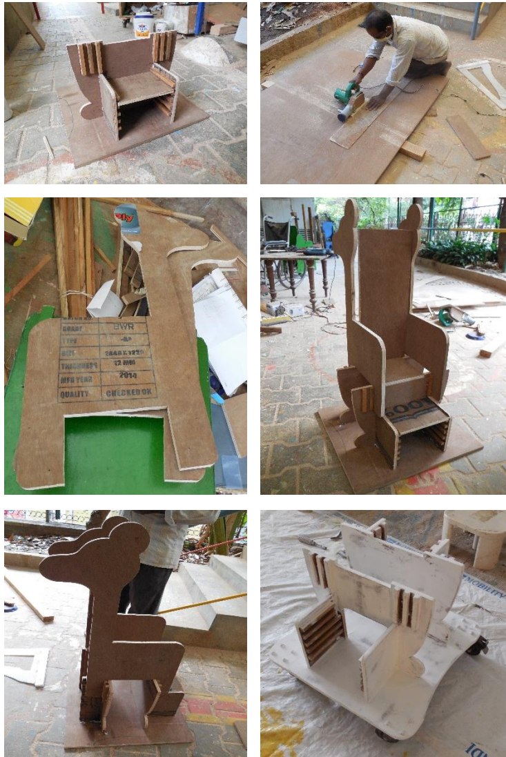
Picture 2 : Prototype being made using plywood Image Source: Author
