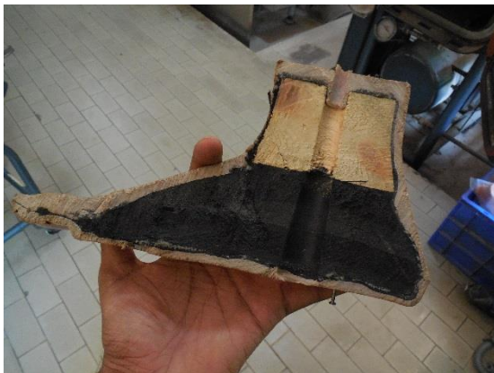
Picture 20. Cross sectional view of Jaipur foot Source : Author
