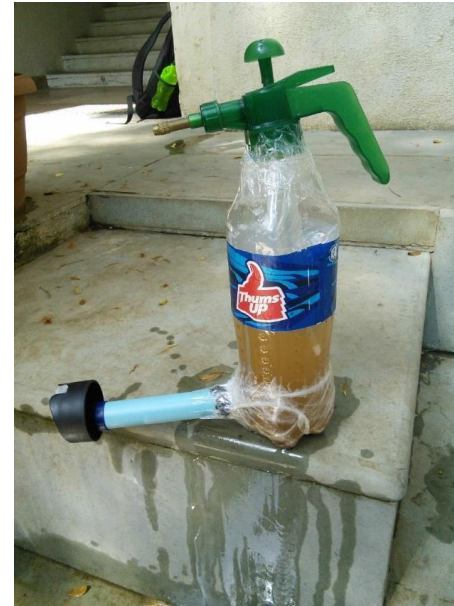
Picture 28: A quick test rig that was done using life straw to test the validity of the concept
