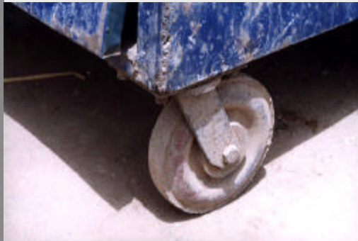
wheel on pivot, difficult to move
