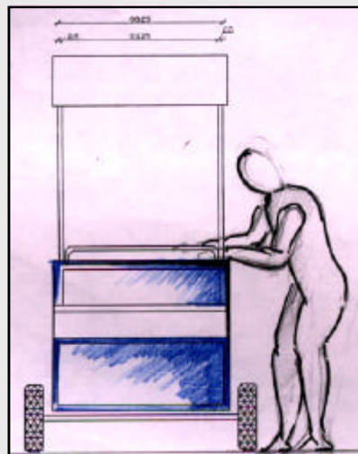
Side ways, front wheel comes under way when cart is used from the sides.
