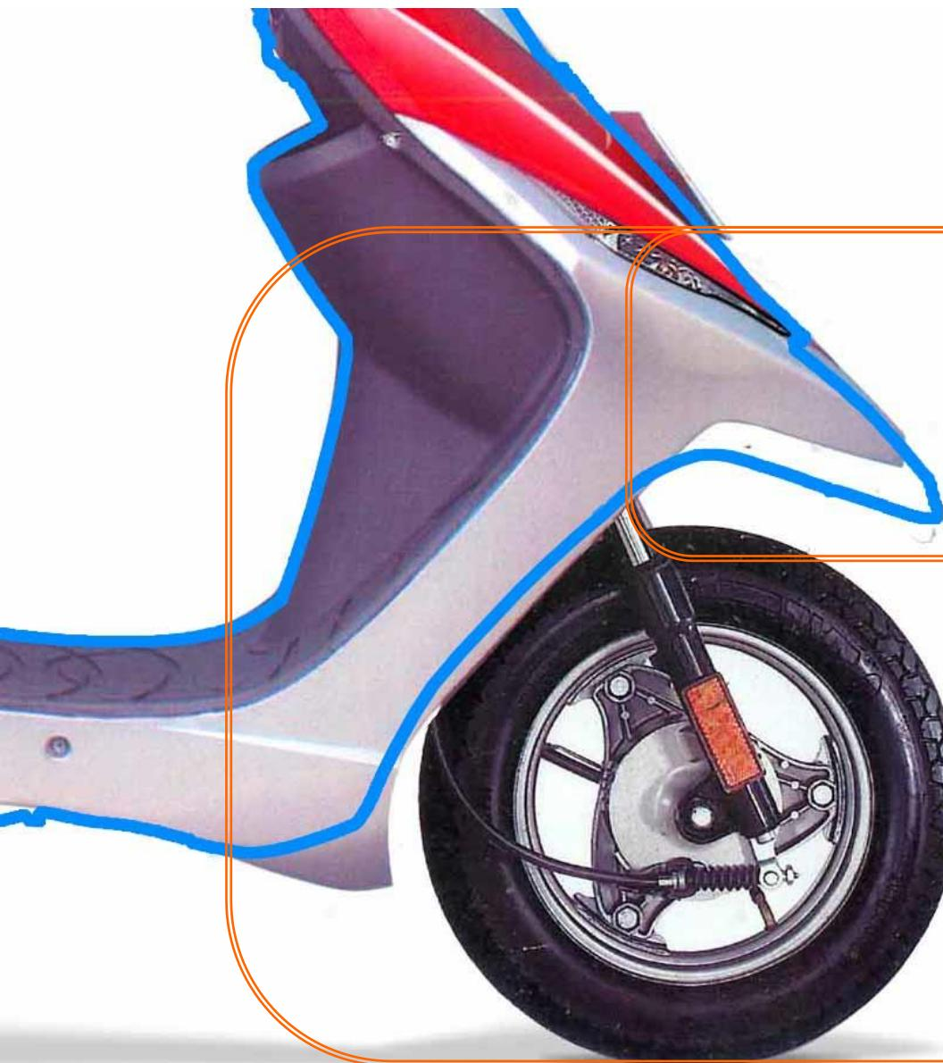
The nose has been cut short by 40mm and even the edge of the wheel well has been treated to add to the over all dynamism.
