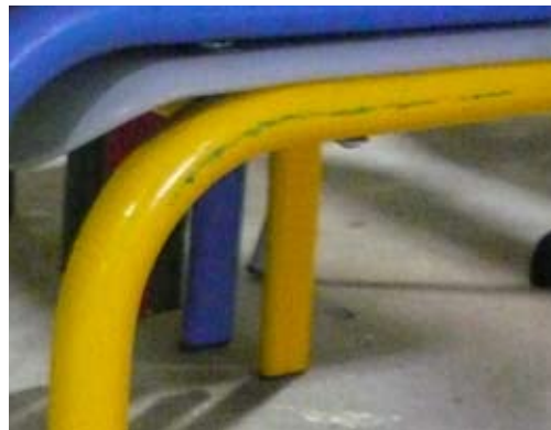
Peeling of paint during stacking of chair
