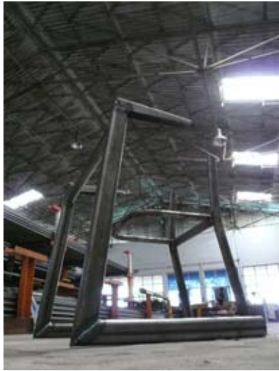
final assembly of frame before powder coat
