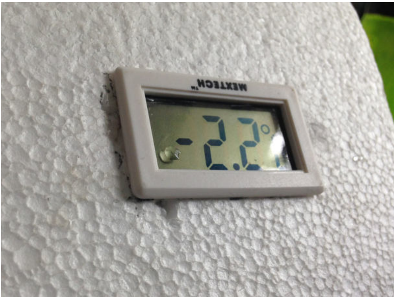
Temperature display showing -2.2 degree celcius from water-cooled peltier
