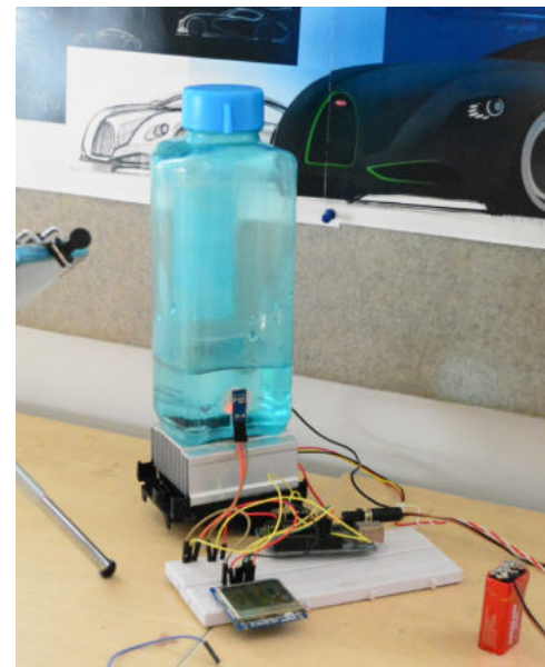
Single chamber with peltier on wall
