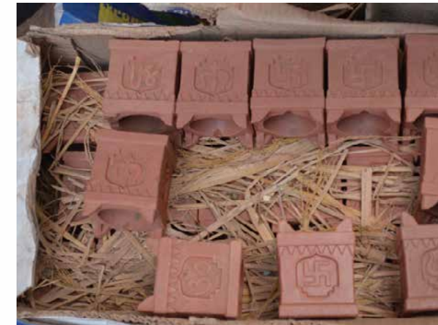
Packaging done using hay between the two pieces
