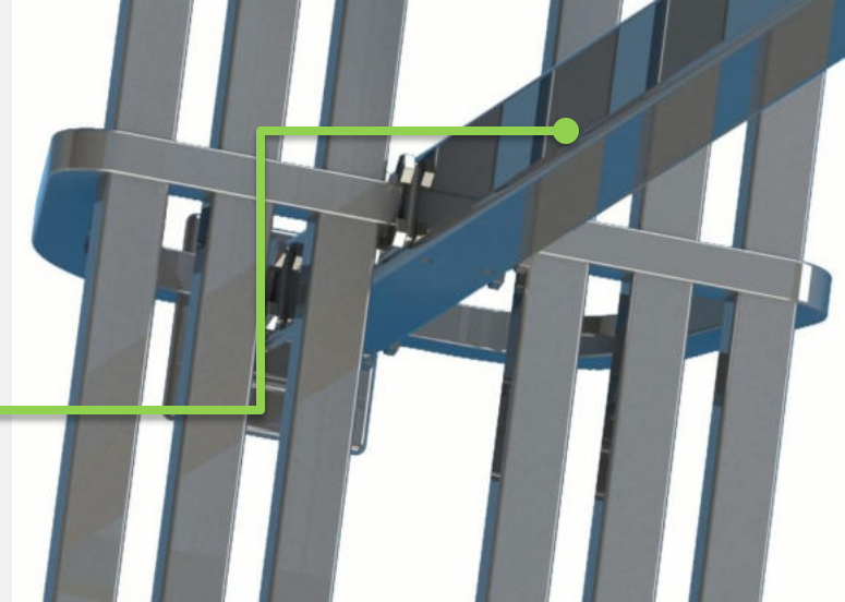
15 * 15 cm rectangular tube stainless stainless steel column
