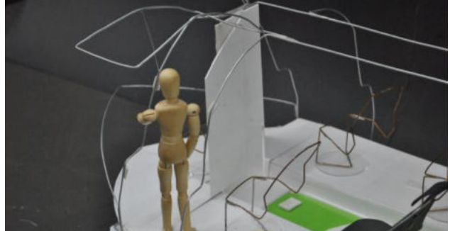
The pictures shows movement of driver from side door to the cabin. One of the side panel slides/folds into middle panel and the middle panel opens to provide room for driver movement as shown in sketch.
