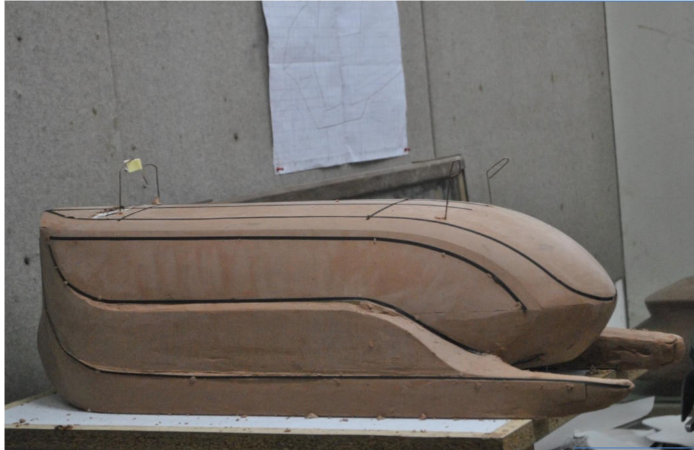
Clay model with roof and window lines.
