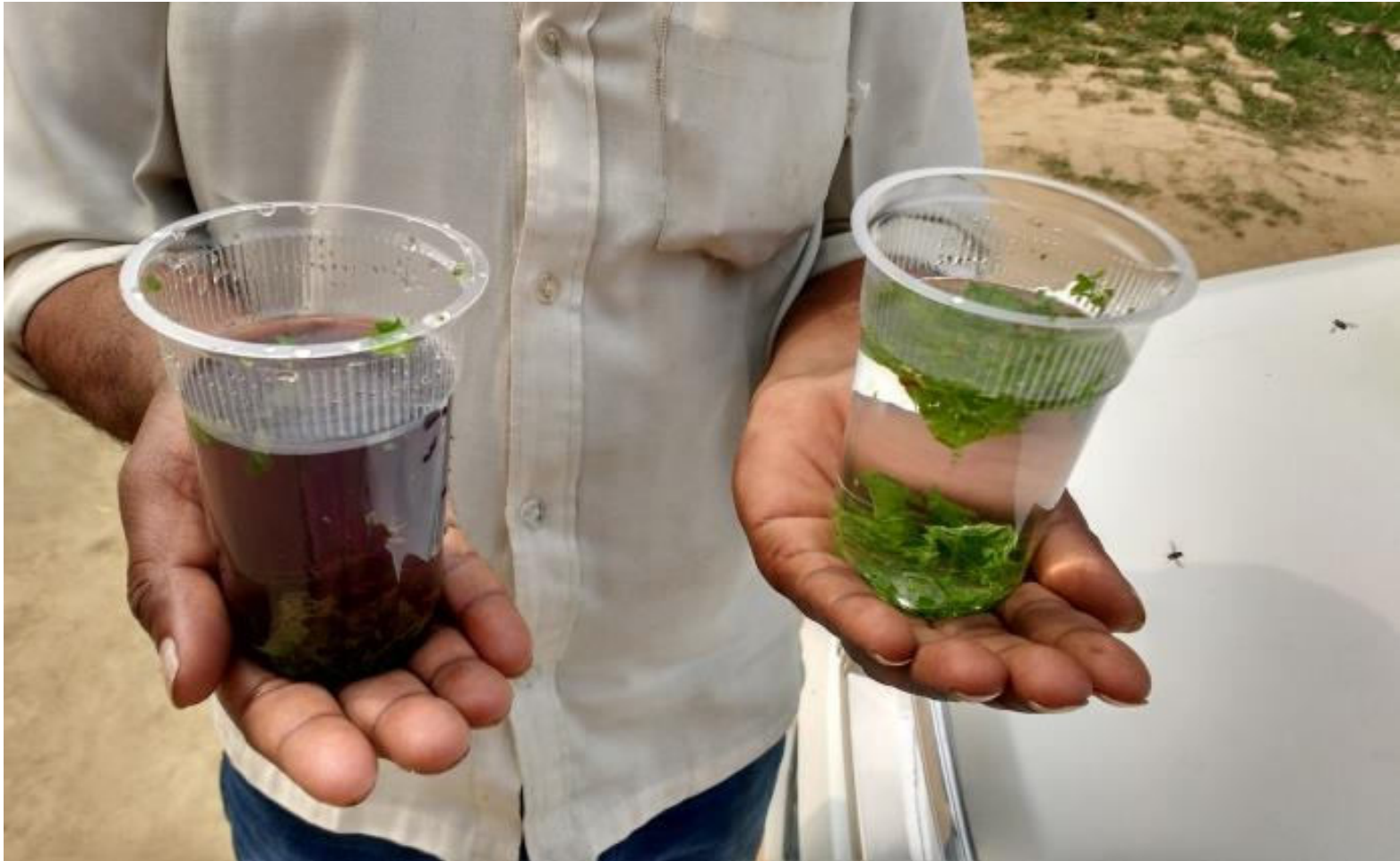
Fig 19: Home based Iron testing is done in villages. Guava leaves are used. The water with higher iron level instantly changes its colour to black when tender guava leaves are crushed and put in it.
