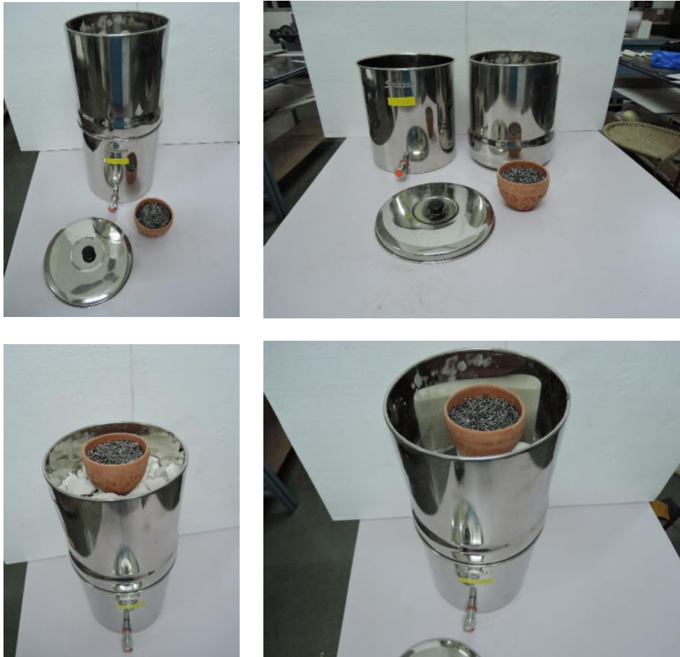
Figure 24: Candle filter modifications to arsenic filter
