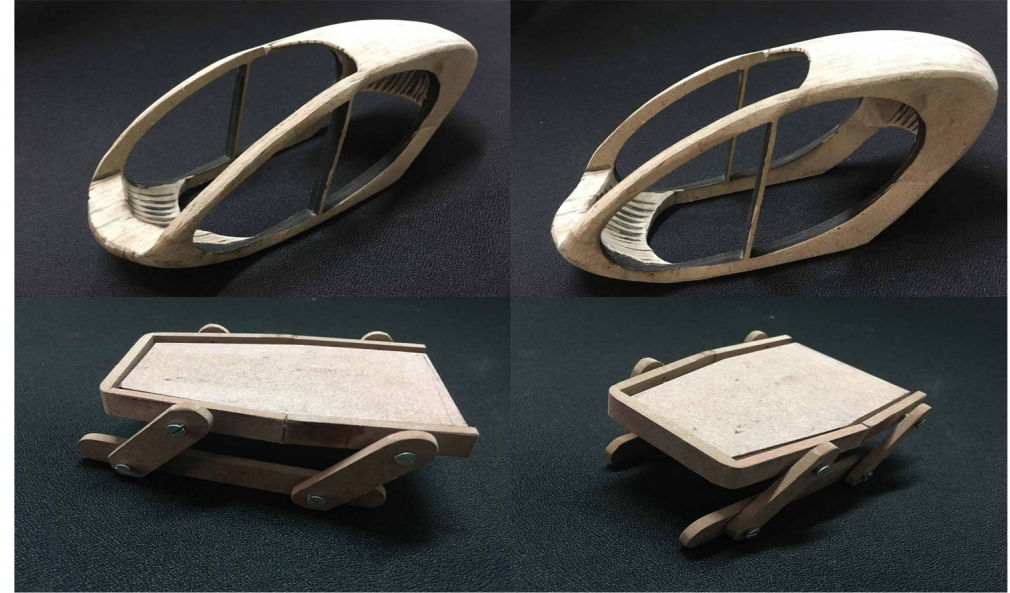
Image 44 : Model - fuselage and Chassis, using mdf to create the basic form of the fuselage
