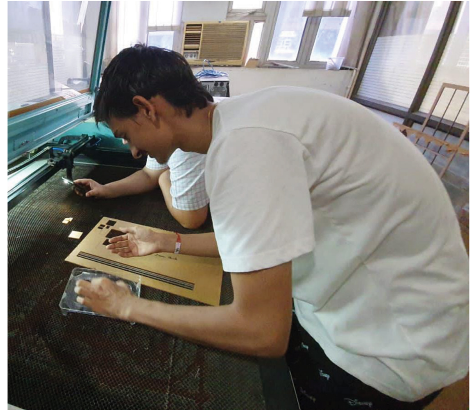
Image 54– Laser cutting of patterns using acrylic sheet
