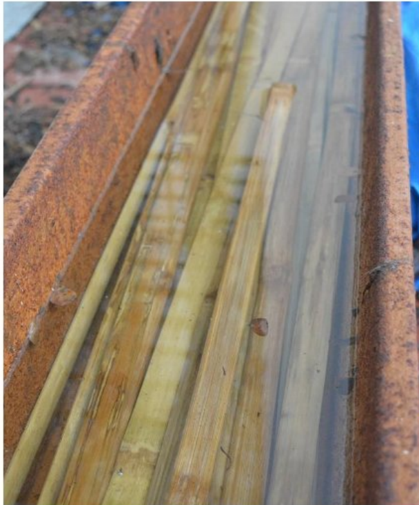
Bamboo slivers kept in water to make it softer for further treatment
