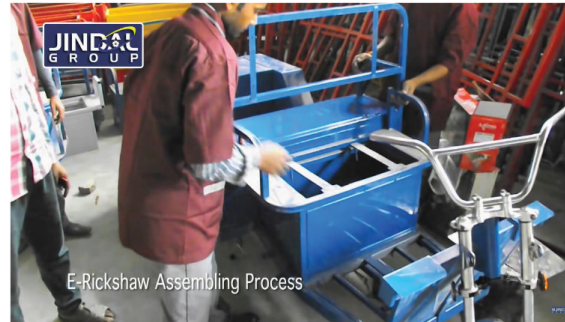
Body assembly (Body on frame)
