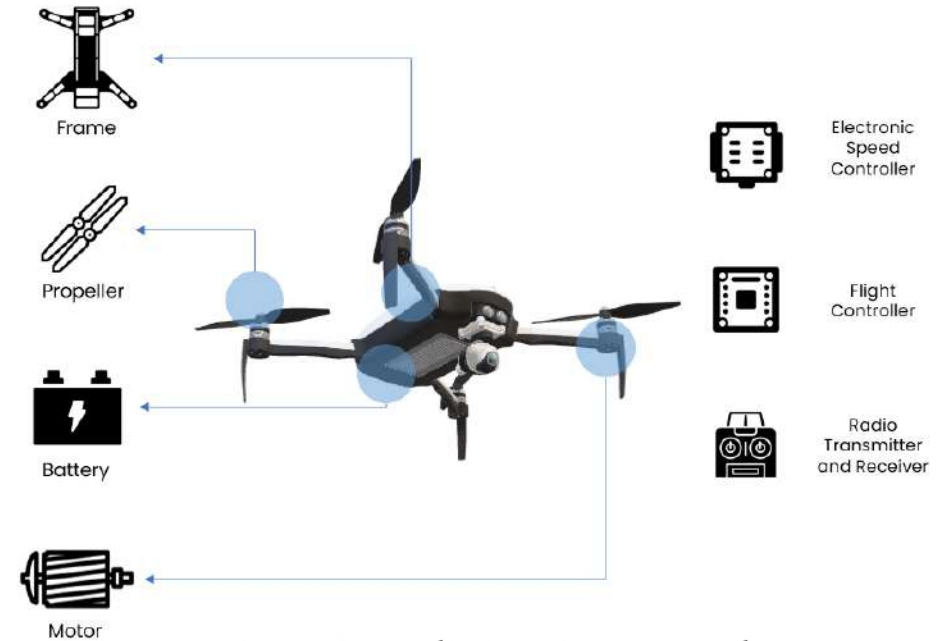
Image 3 : Drone Architecture Image source : Author
