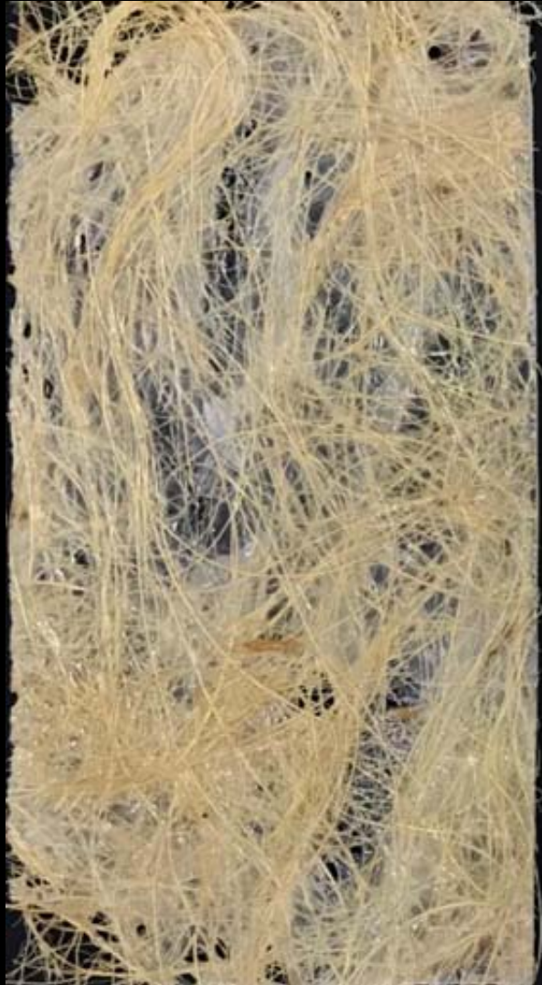
10. Coir- Long fiber in epoxy resin (sprinkled with water for translucent finish)
