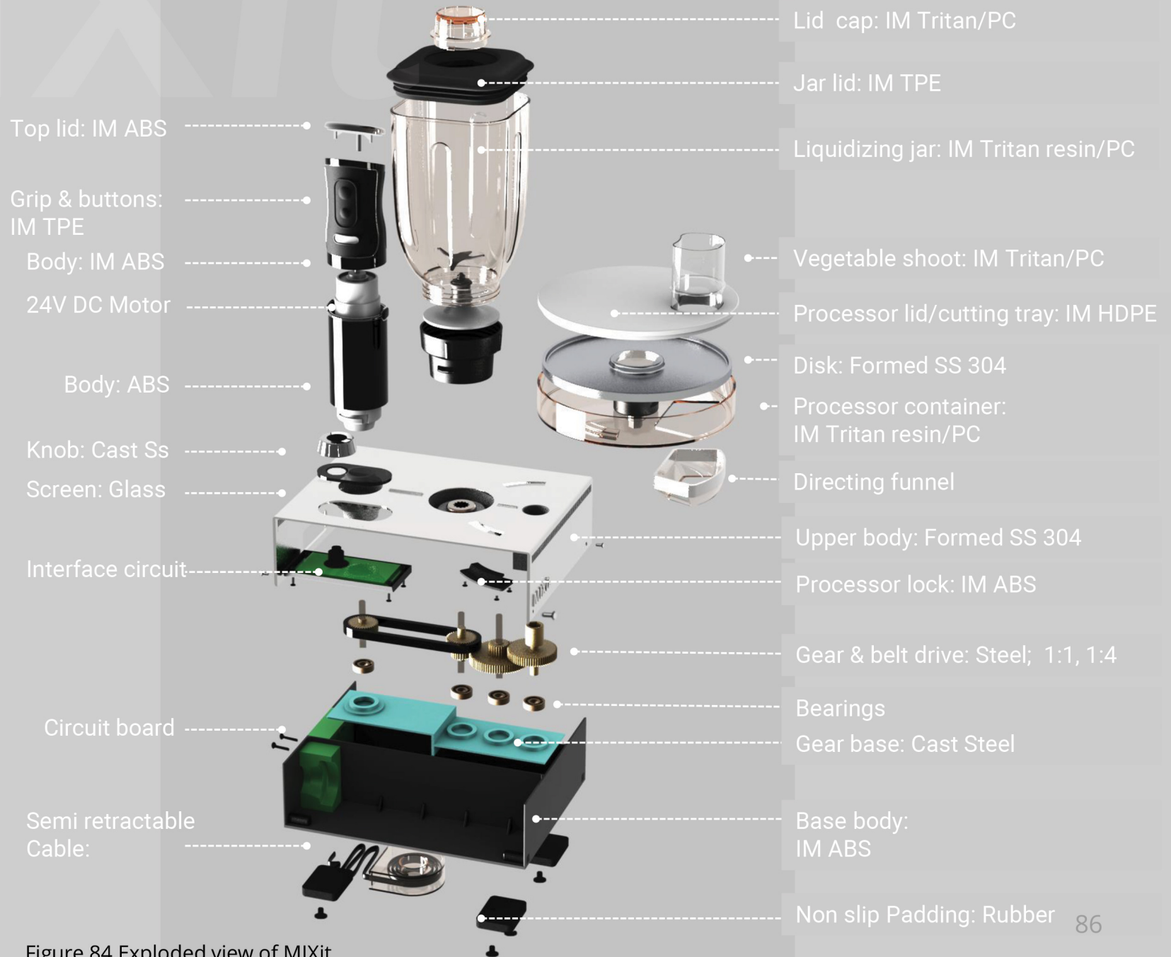
Figure 84 Exploded view of MIXit
