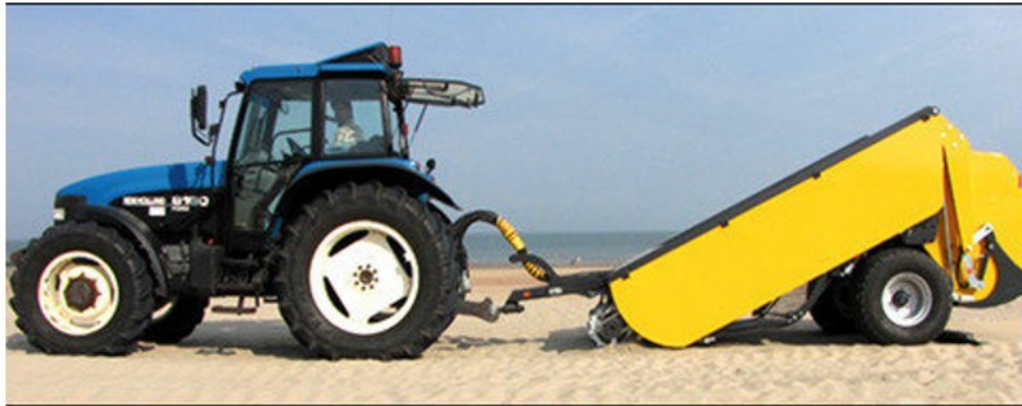
Image 19: Combined Sifting and Raking machine (pull type) - has a roller which rakes the sand, then a screen sifts the sand down and the hopper collects the trash.
