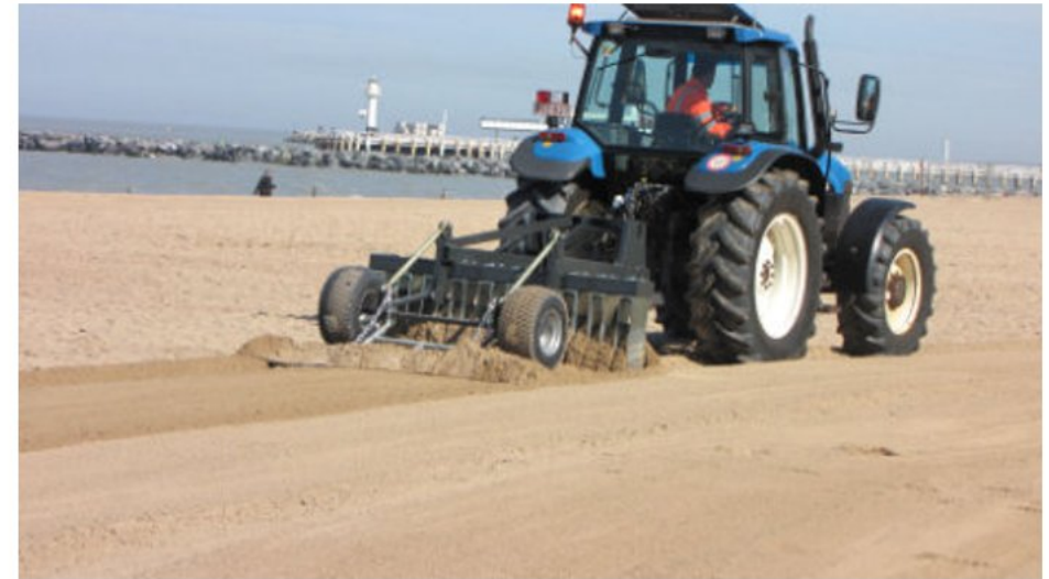
Image 21: Heavy pressure rake (pull type) used to turn the sand.
