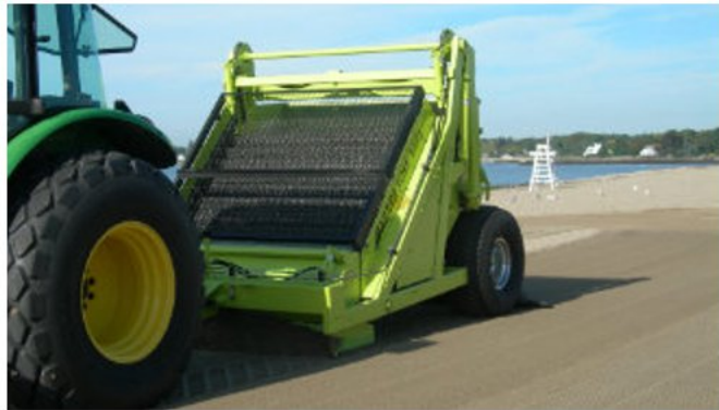
Image 17: Sand raking machine
