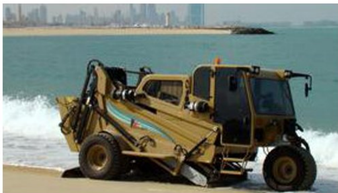
Image 18: combined sifting and raking machine
