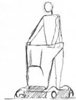
Idea for a stan-over mini cleaner that user body weight pressure and forward motion for turning the mechanism
