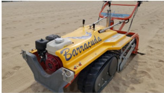
Image 16: Sand sifting machine
