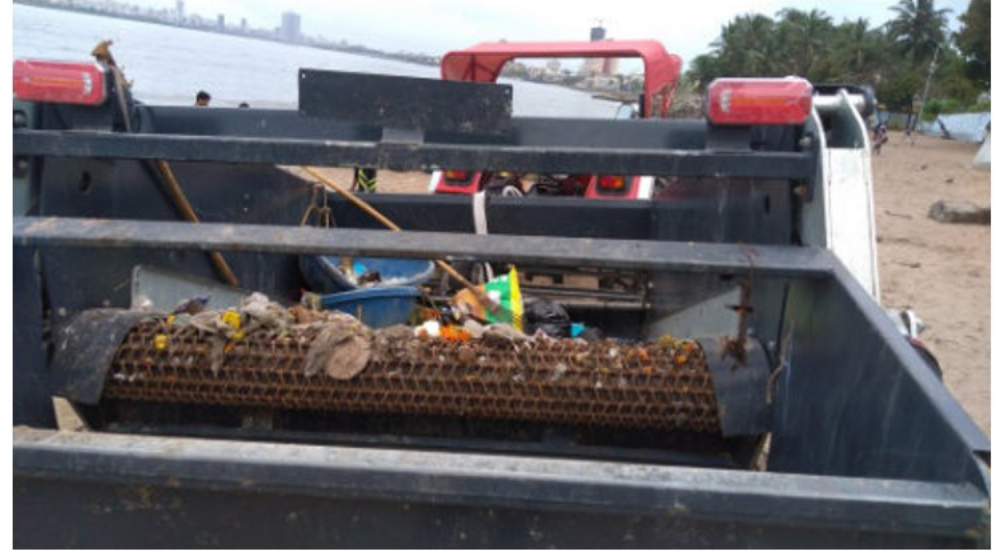
Image 47: In a disorganized way manual cleaning equipments are always kept. In this case they are kept in the screen itself which is contaminated and harmful.
