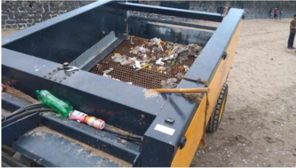
Image 46: Machines cannot differentiate what they are picking. Clog on the screen.
