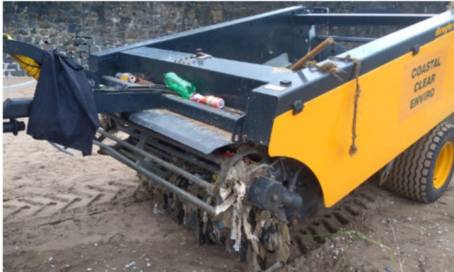
Image 44: Clogged trash picking machine at Dadar
