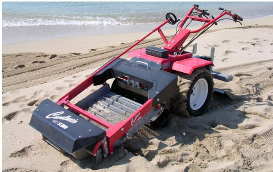
Image 20: A walk behind sand sifting machine which screens sand and is very maneuverable and easy to operate.
