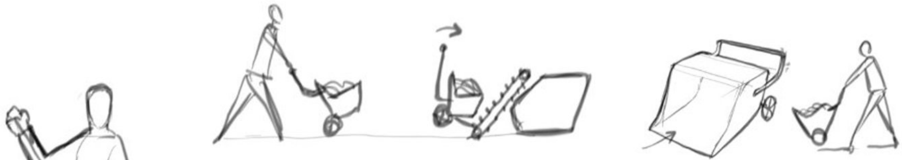
Idea for manual scraping and carrying. Assistance of a mobile compactor and hopper. Human and machine.
