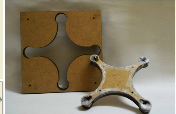
Construction of the mold using Inventor as drawing software and MDF as base material
