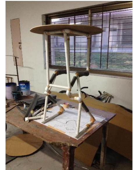
Figure 21.1:1 final prototype made from pvc pipes
