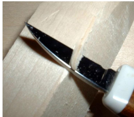
fig 2.39 Shaving Slivers of a wood
