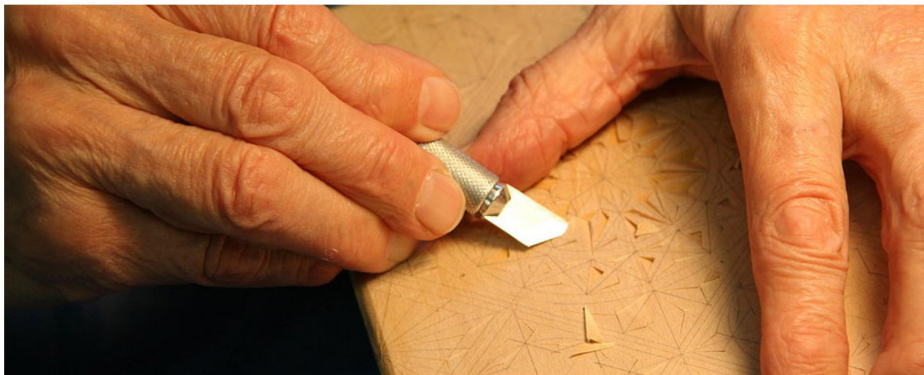
fig 2.35 Chip Carving using Knife tool
