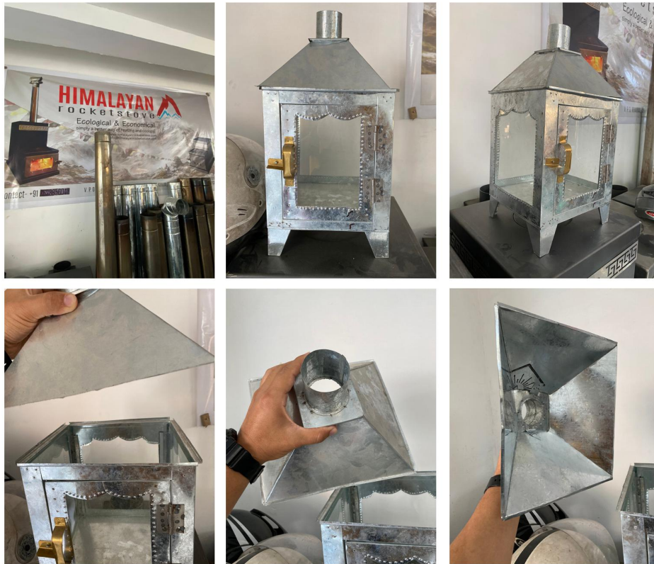
fig 2.41 Chukun Chomey stand made up of steel sheet
