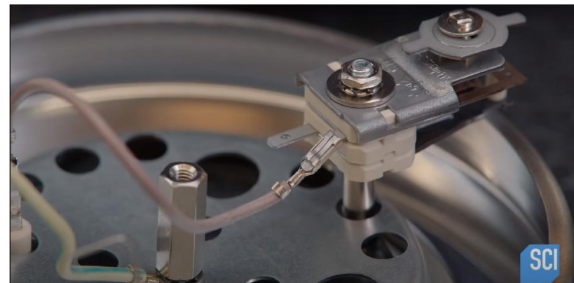
Image 4.11. Thermostat used in hotplates.
