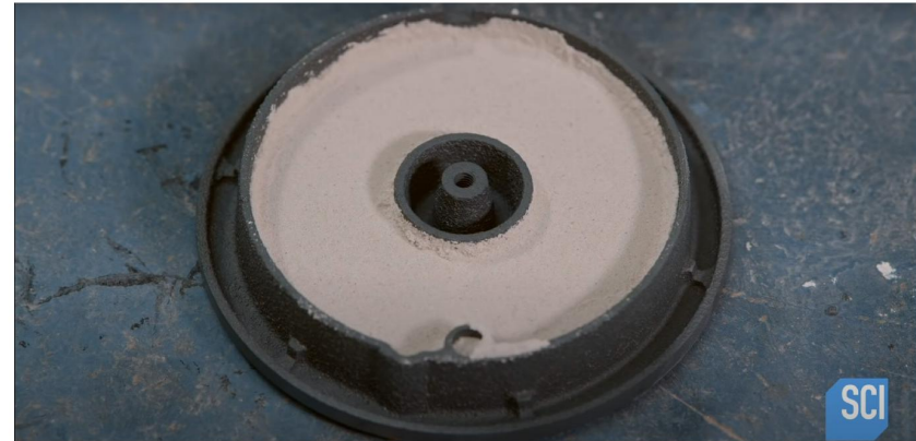
Image 4.10. Insulation used in hotplates
