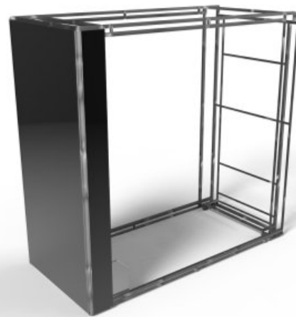
FRP/aluminium sheet with form inside
