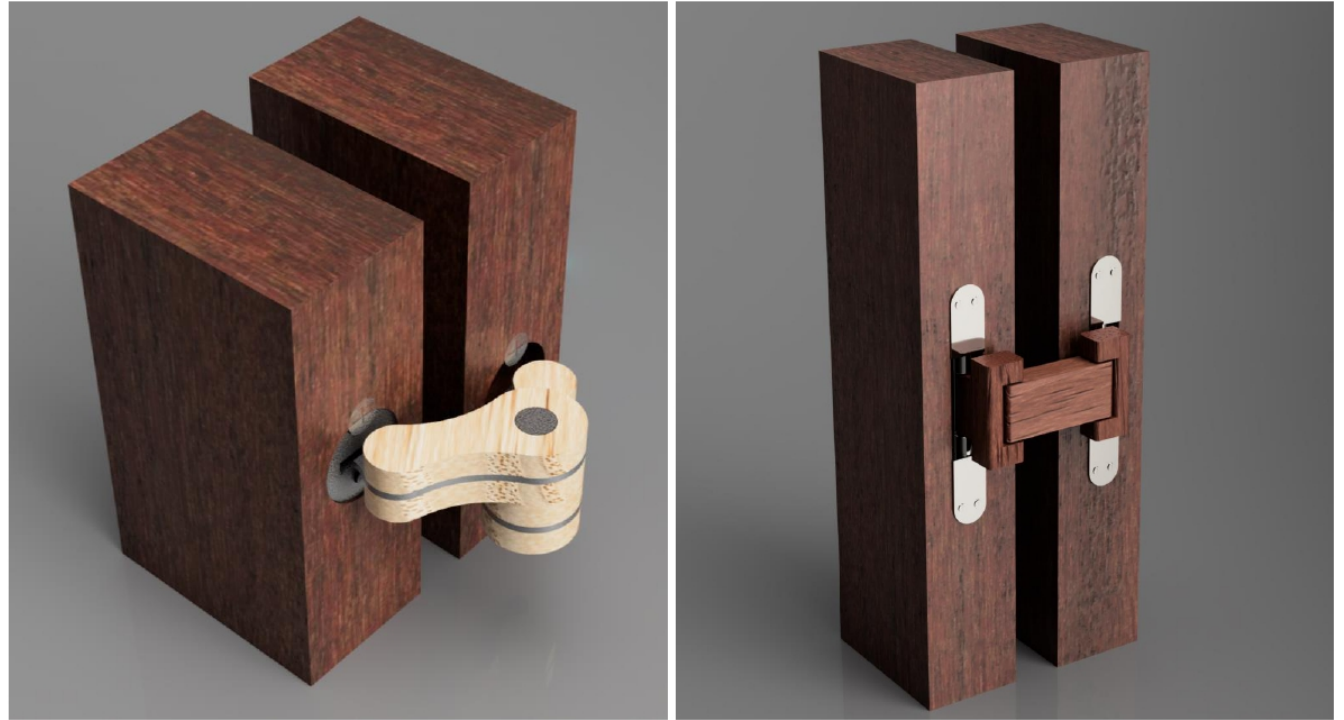
Fig 118: Hinge detail (for wood) Source: author
