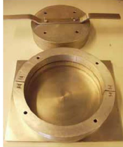
Fig 15: Mould in which coconut husks are hot pressed to produce fibre boards. Source: [IR3]
