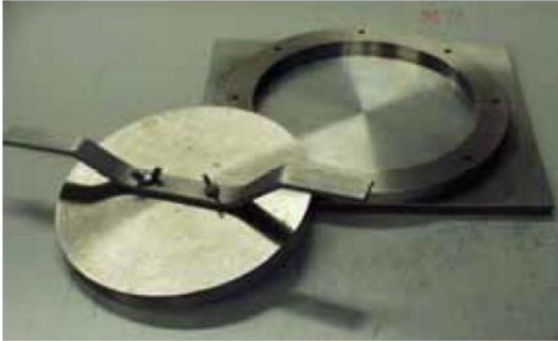
Fig 15: Mould in which coconut husks are hot pressed to produce fibre boards. Source: [IR3]
