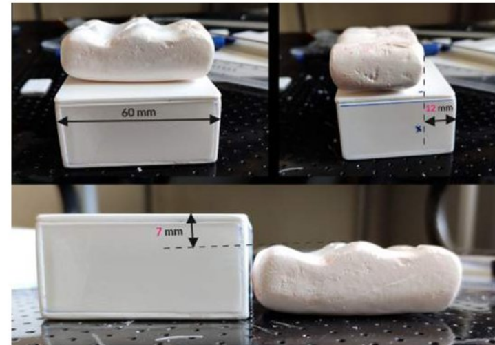
Figure 70: Image shows the overshoot of dimensions of pre-final prototype from the proposed product.
