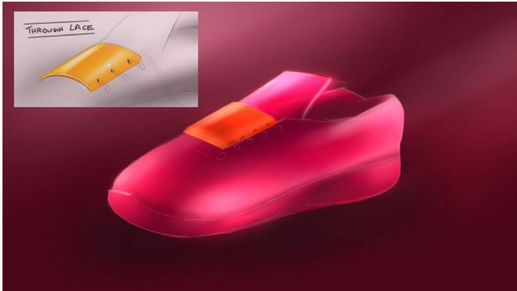
Figure 24: Non-photorealistic rendering of the product (orange colored) tied by the lace of the shoe. The image on the top-left shows the visible holes near to the base of the product, that allows it to lace with the shoe.
