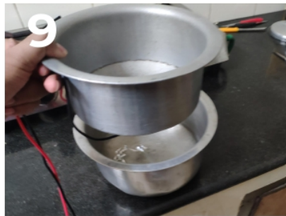
9 Inner pot with Filament is placed inside the vessel with PCM.
