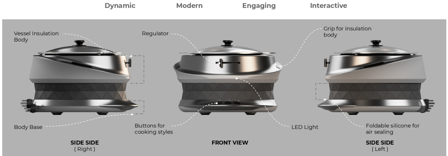
Figure 49 : Renders showing elevations of the final design
