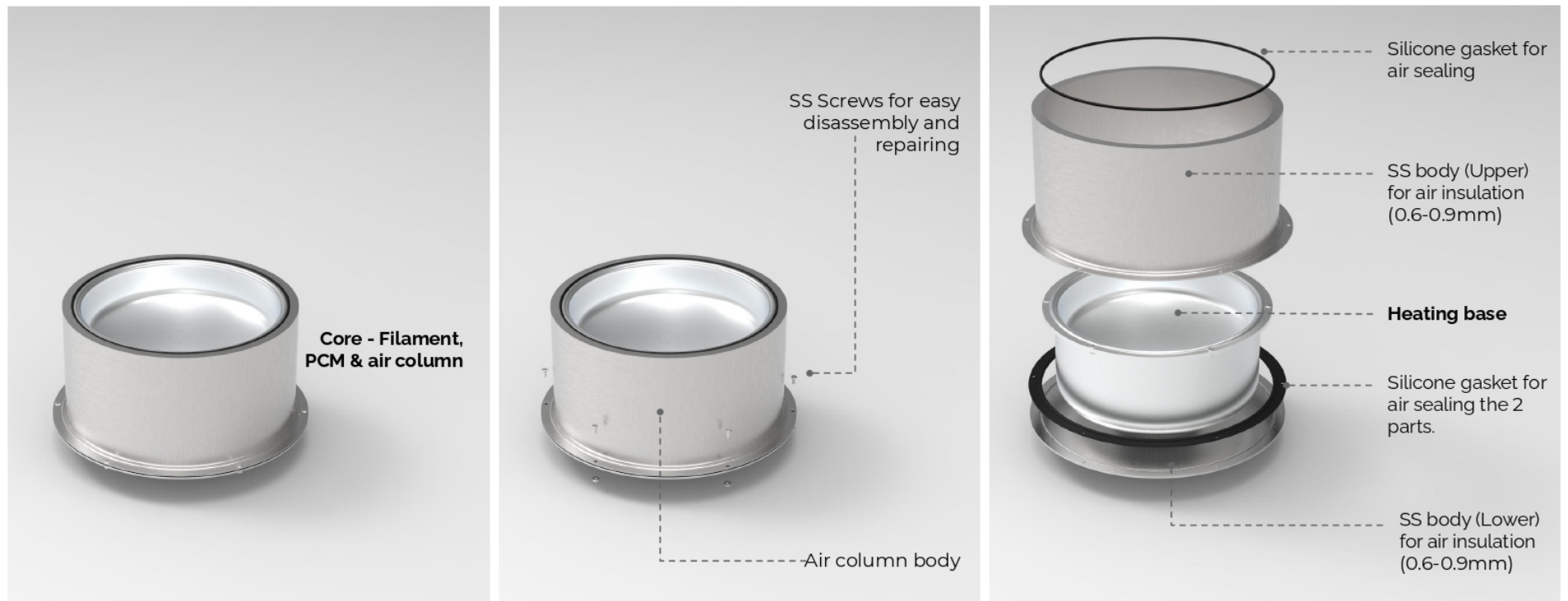
Figure 82, 83 & 84 : Steps to open outer body of the core for easy assembly / repairability.
