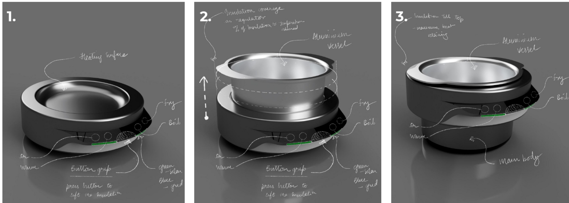
Figure 41 , 42 & 43 : Renders showing working mechanism of exploration 01; 1 is default position, 2 vessel kept on stove and 3 insulation slid over the vessel.
