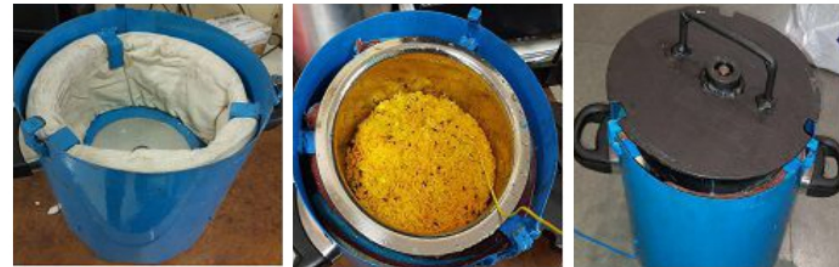
Figure 17 : Vessel with polyurethane insulation jacket
