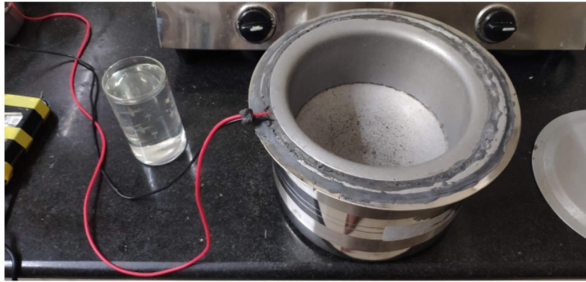
Figure 26 : Testing the rig - Preheating the vessel
