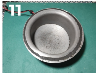
11 Inner pot retains the position after the PCM solidifies. All gaps are sealed so that PCM does leaks out.
