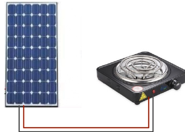
Solar ( DC power ) - Resistive coil ( Heat )
