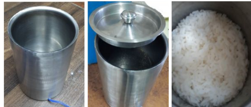
Figure 18 : Double walled cookstove with trapped air acting as an insulation
