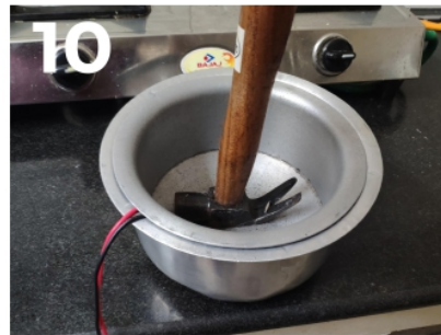
10 Weight are put on the inner pot to counter the buoyancy from the PCM and left until PCM solidifies.
