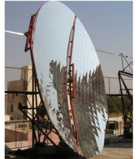
Solar steam boiler
