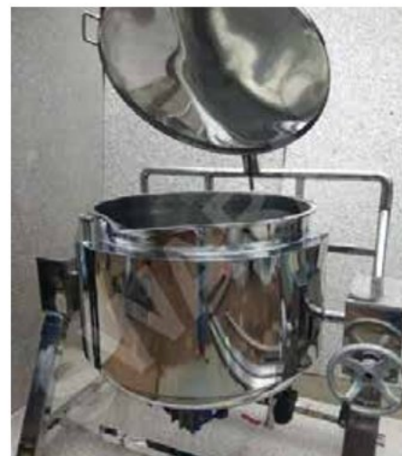
Fig12. Steam kettle with stirrer and packaging.
