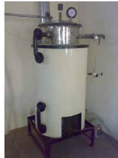
Fig6. Fire wood steam boiler
