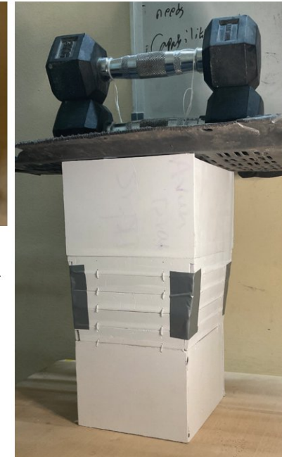
The assembled mockup is load tested with 6kgs dumbbell on top of it.
