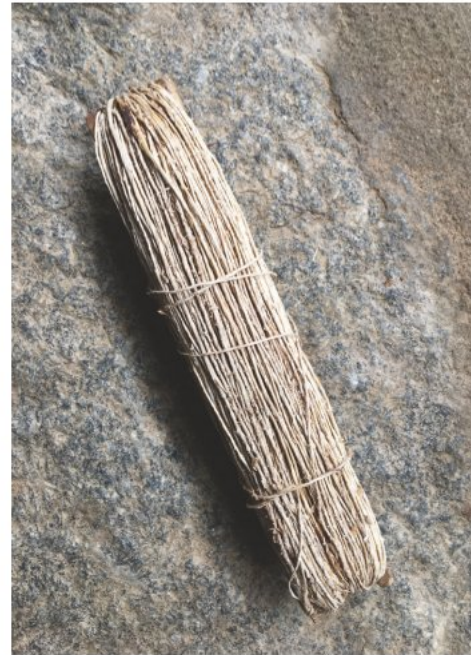
Banana fibre rolled up in a shuttle to get used as weft for weaving
