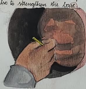
**Soldering:** The parts of the product are made separately and then joined together. These jointed parts are soldered. For joining a powder (made of sinkha, jasta, palat, kansa roong and naurasda) is mixed with water and applied on the jointed areas. The product is again heated on furnace then allowed to dry.
