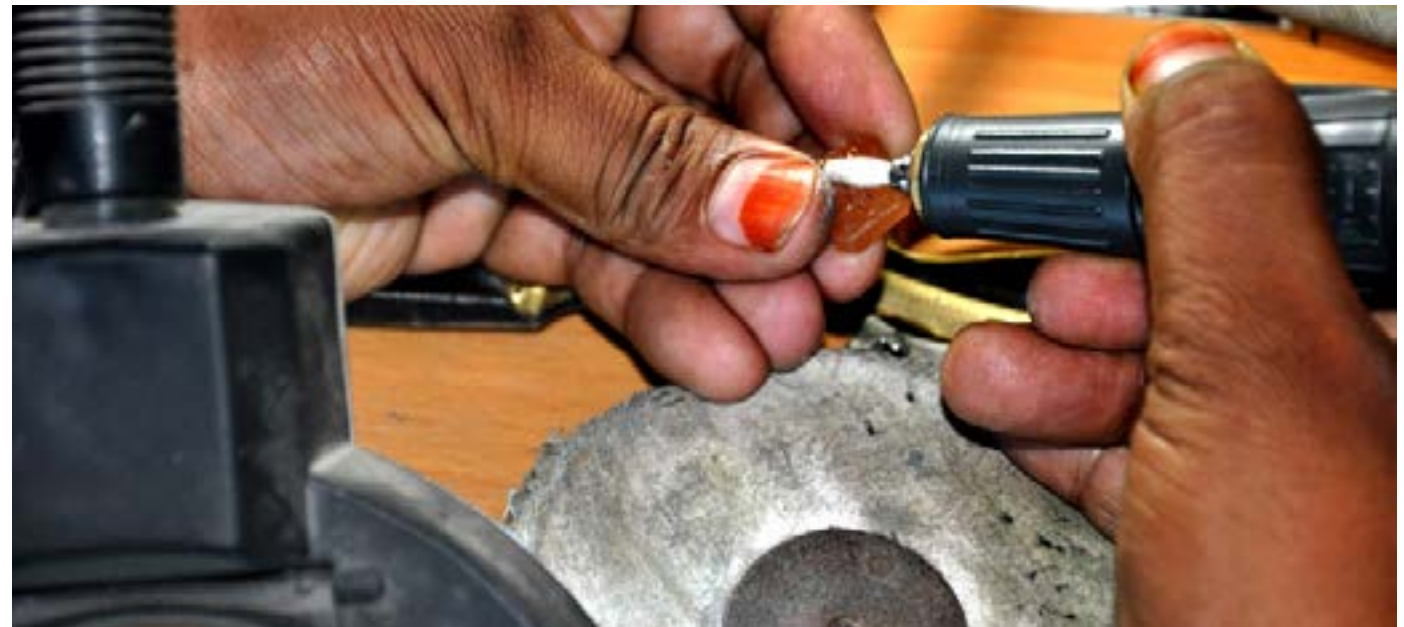
Creating the script on stone using automated drilling tool.
