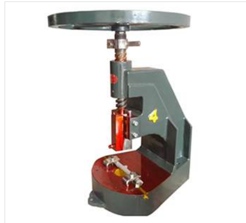
Hand operated Fly Presses are available with tonnage up to 5 T. (Image source)
