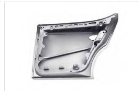
Resistance welded automobile door. (Image source)
