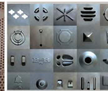
Different punch operations without removing the sheet from machine. (Image source)
