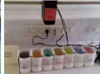
A mini PLC controlled 7 tank process. (Image source)
