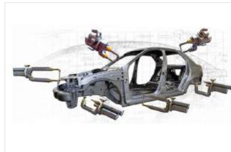
Extensive use of spot welding in automobile bodies.
