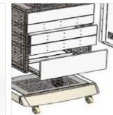
A Medical Cart uses "push to open" slides to open the drawers, eliminating protruding handles.
