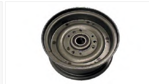
The nuts on the wheel hub are projection welded.
