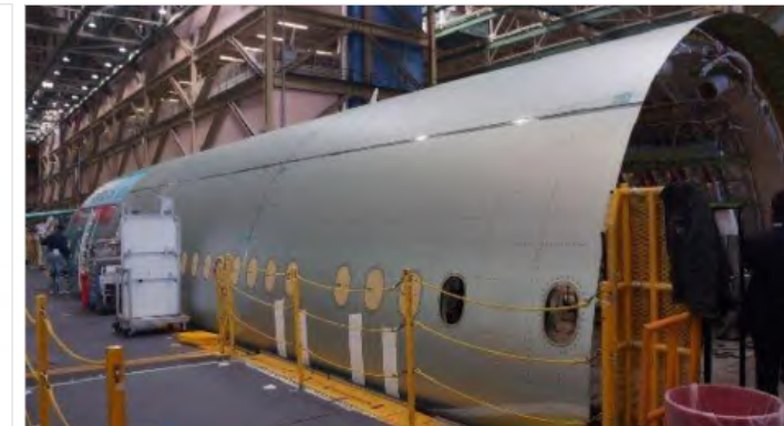
Aircraft fuselage by stretch forming. (Image source)
