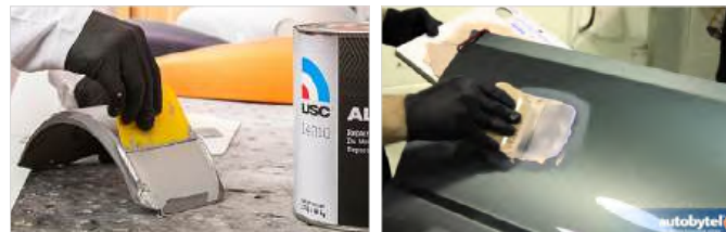
Application of putty with blade. (Image source)
