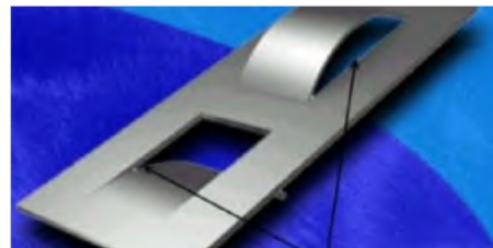
Pierce and Plunge - To produce in-built hooks and Handles.
