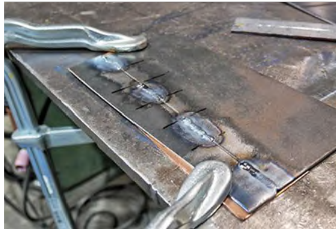
Skip welding. Skip and weld ( Image source )
