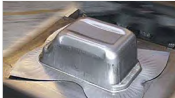
Deep drawn part before trimming.
