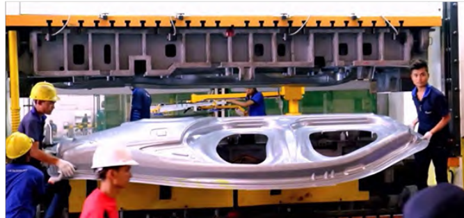
A 2000 Ton press used for an auto body part forming. (Image source)
