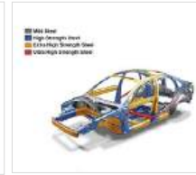
Different grade of steel in au- tomobile body. (Image source)
