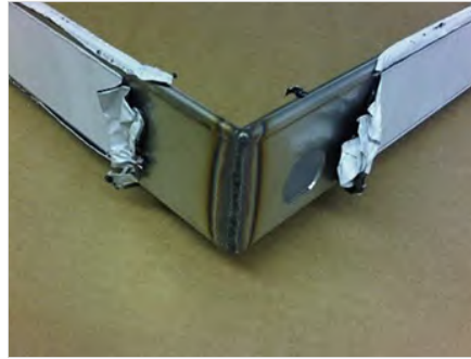
Direct corner edge welding. (Image source)
