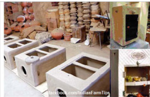
Mitticool – A clay refrigerator
