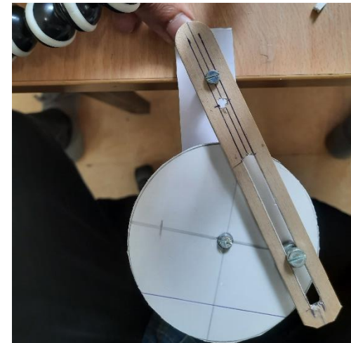
Fig 5. Desirable motion for the toy (left), quick mockup for the mechanism to mimic the desired motion (right)
