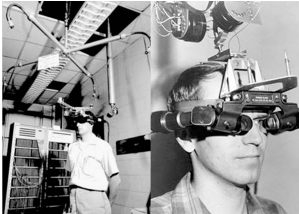
Fig 1. Ivan Sutherland's first VR Head Mounted Display, The Sword of Damocles Image Source
