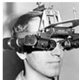
The Sword of Damocles - Head Mounted Display
